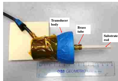
Figure 6. Vibration delivery structure: substrate rod.
