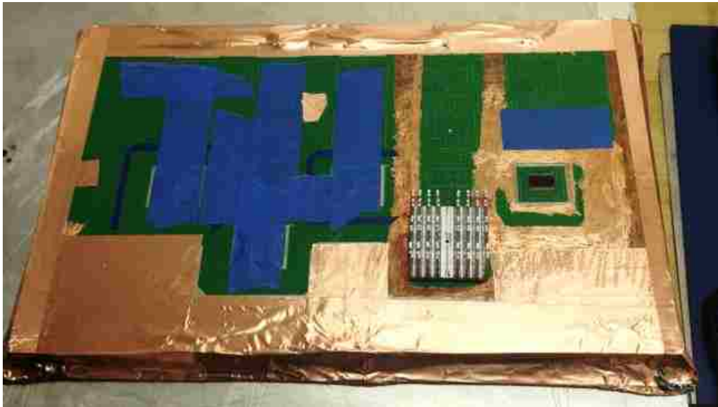
Figure 5.3. Clock buffer IC board for validation
