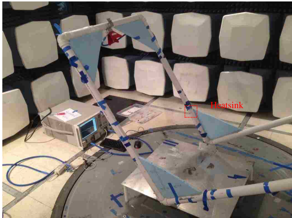
Figure 4.1. Maximum far field measurement setup
