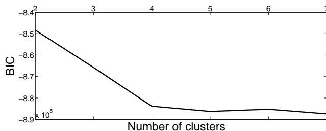
Figure 4: Cluster validity using BIC. After clustering into k clusters using spectral clustering, the partition BIC calculated using (9) is used as a cluster validity index. Higher index indicates better partitioning.
