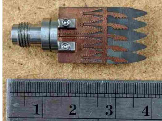
Figure 6. Fabricated antenna with the middle element being fed while the other four are left open.
