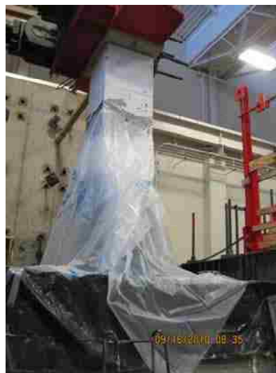
Figure A.8. Curing of the CFRP System
