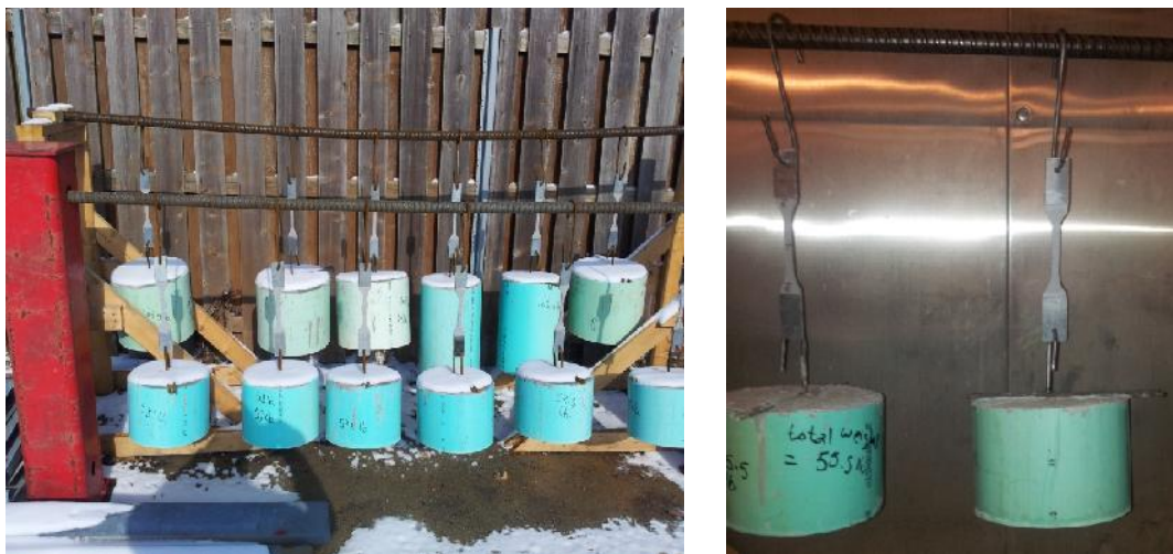
Fig. H-28. Sustained stresses together with natural thermal cycles (left image) and computer controlled thermal cycles (right image)
