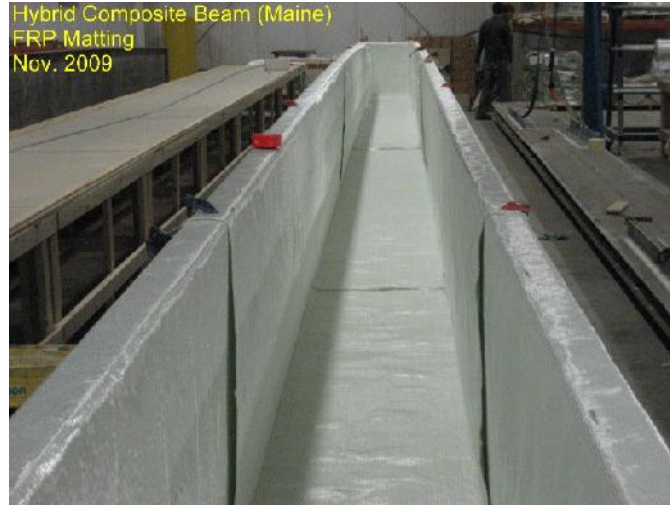
Fig. A-1. Layup of the GFRP shell
