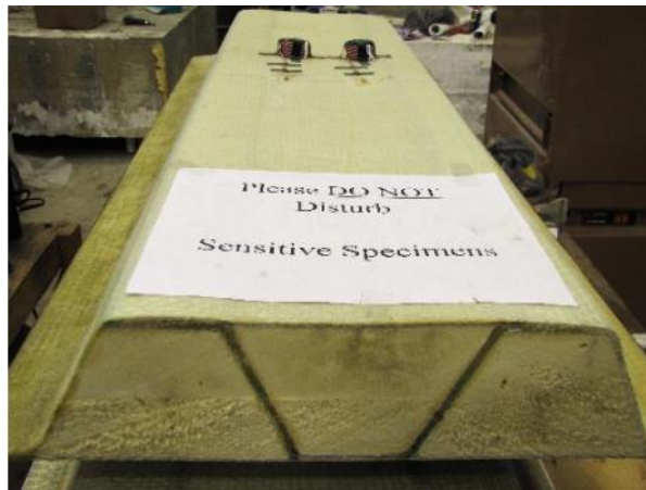
Figure 1.10. GFRP sandwich deck panel (Tuwair et al., 2014)
