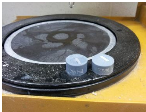
Fig. H-6. Samples' polishing via mechanical polisher
