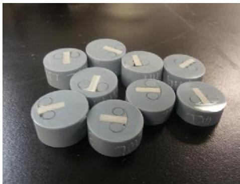
Fig. H-7. Polished samples by 1 micron monocrystalline diamond solution.
