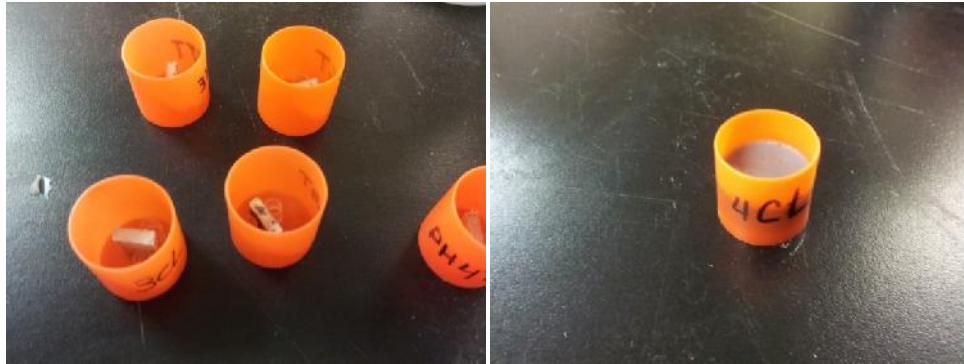
Fig. H-5. Samples' mounting with Varidur epoxy
