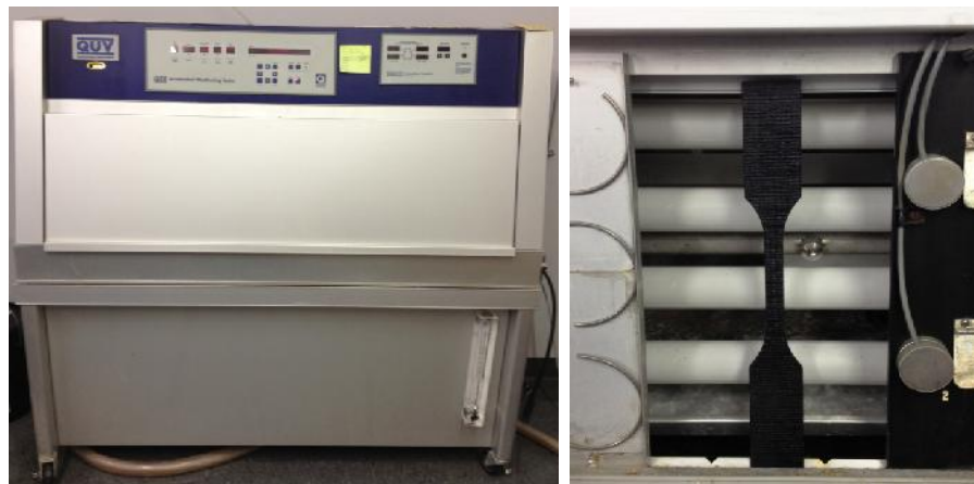
Fig. H-24. UV-irradiation apparatus (Left image) GFRP specimen exposed to UV-irradiation (Right image)
