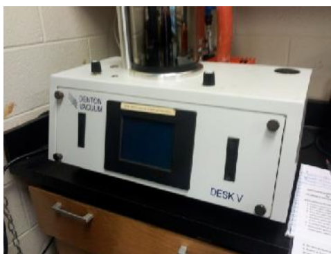
Fig. H-8. Sputter Coater Device
