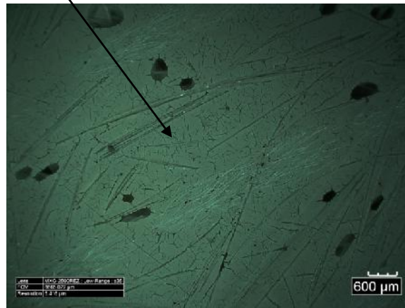
Fig. 22. Formation of micro cracks in the surface of uncoated specimen (2L-UV-SF) following UV
