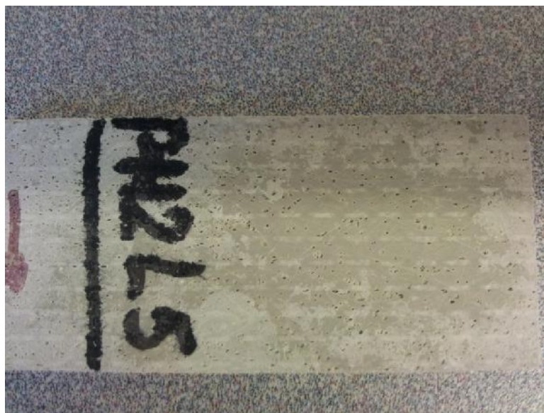
Fig. H-38. Camera image shows the voids on the exterior surface of 2L-Alk specimen
