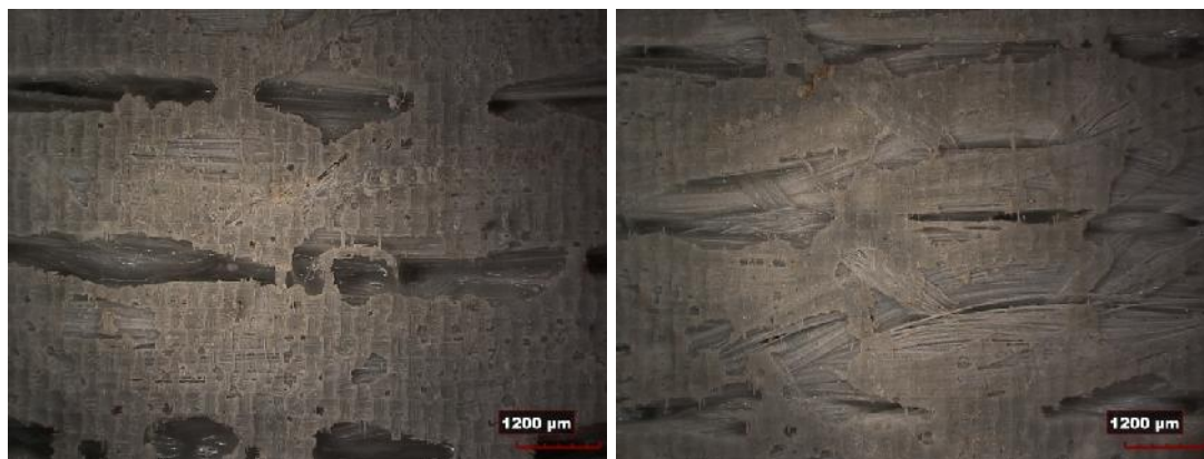
Fig. H-36. Existing voids in unconditioned specimens' interior surface
