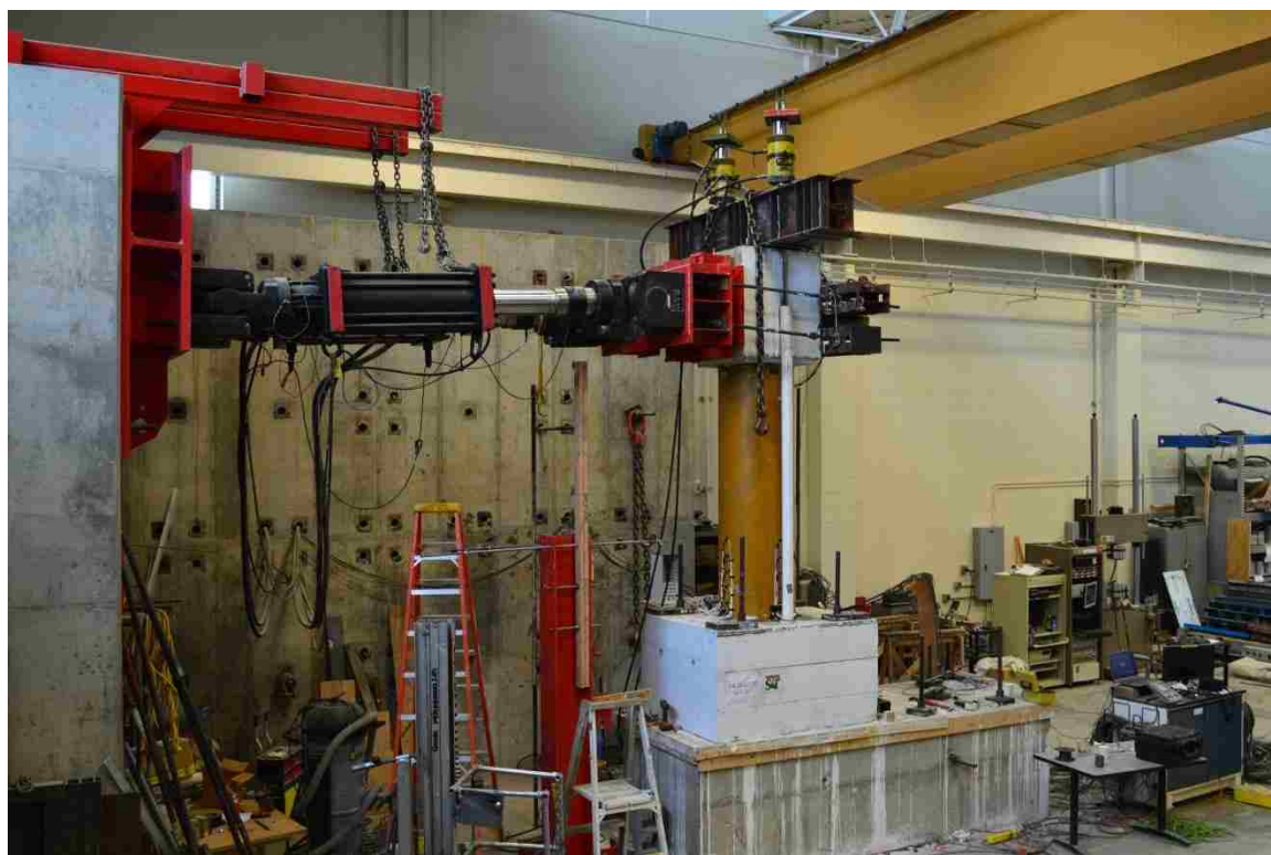
Figure B.17. Large-scale column test setup
