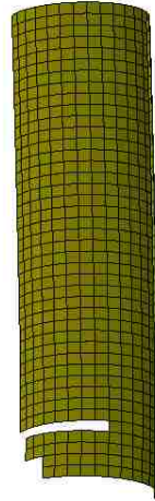
Figure 11. Rupture of the FRP tube during the FE
