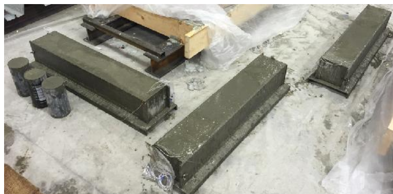
Figure 7.3. RC beams and cylinders for corrosion test.
