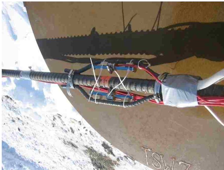
Figure 5.19. Attachment of Strain Gages (Step 5)
