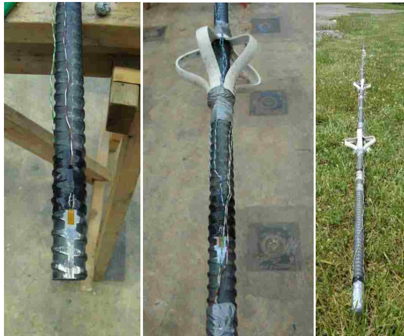
Figure 3.3. Ber Juan Load Test Instrumented Center Bar
