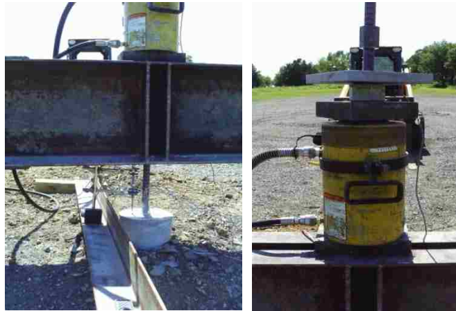
Figure 3.2. Ber Juan Load Test Instrumentation Location
