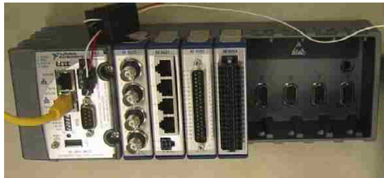
Figure 3.14. CompactRIO Controller and Chassis with Four Modules Installed
