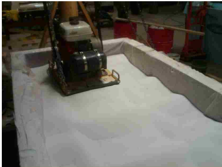
Figure 4.13. Photograph of Sand Placement using Vibratory Compactor
