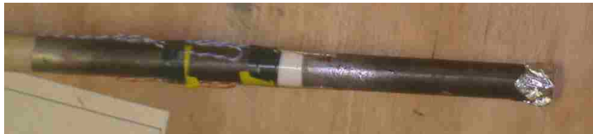
Figure 4.19. Photograph of Micropile End Cap (Step 1)
