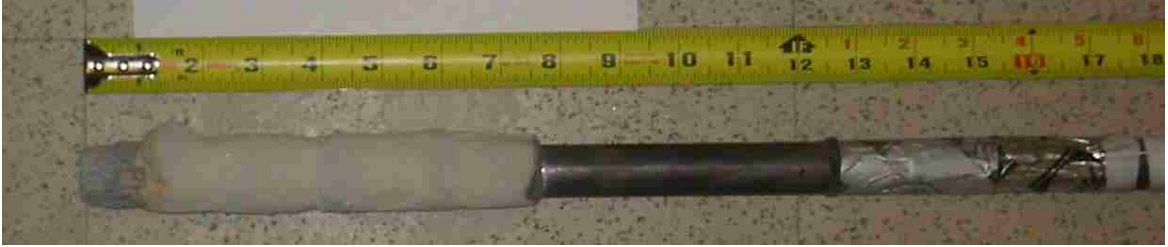
Figure 4.28. Photograph of Exhumed Pile 3D Bond Zone
