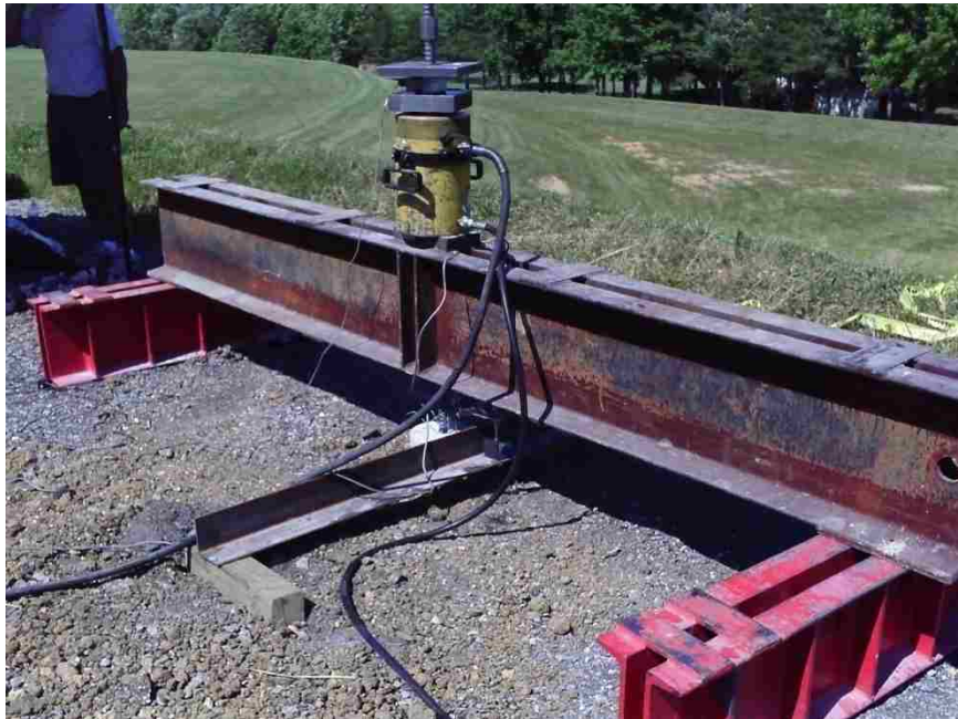
Figure 3.4. Ber Juan Load Test Setup
