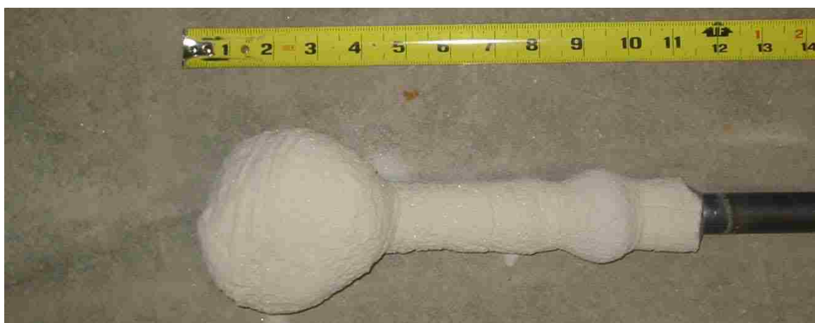
Figure 4.27. Photograph of Exhumed Pile 2B Bond Zone
