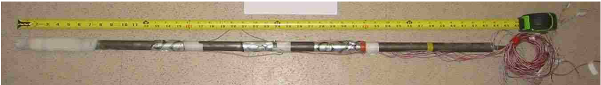
Figure 4.29. Photograph of Exhumed Pile 3B
