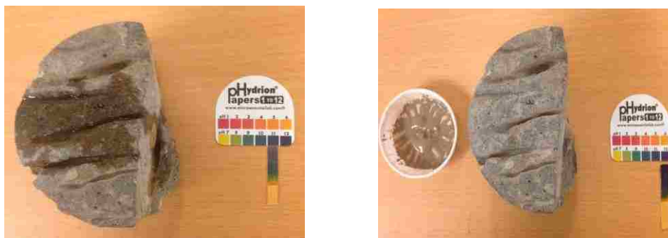
Figure 5.72. pH measurement (Sierrita de la Cruz Bridge): ASTM F710 (left) and Grubb's method (right)
