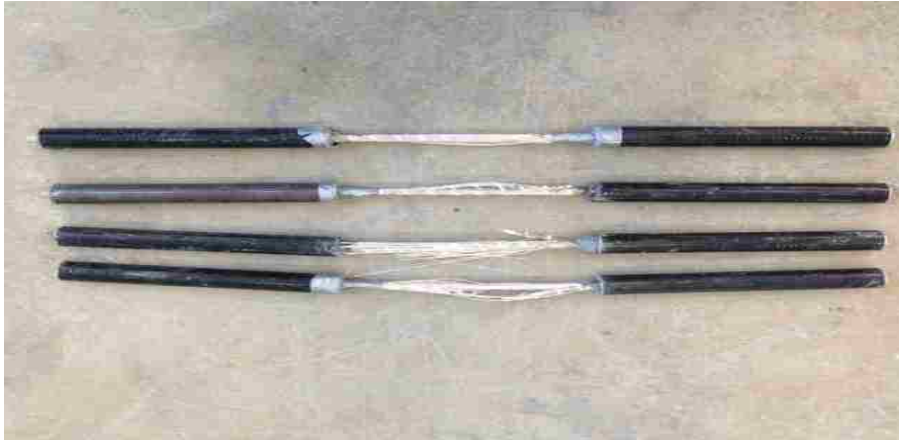
Figure 3.13. Failed specimens of GFRP Bars
