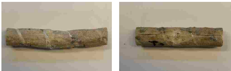
Figure 5.42. Failure #5 (left) and #6 (right) GFRP bars from Sierrita de la Cruz Bridge
