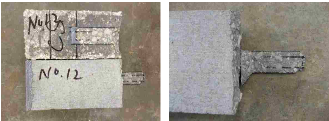
Figure 4.27. The failure mode of a representative control specimen reinforced with galvanized coating steel fibers (RG 7, Failure Mode 1)
