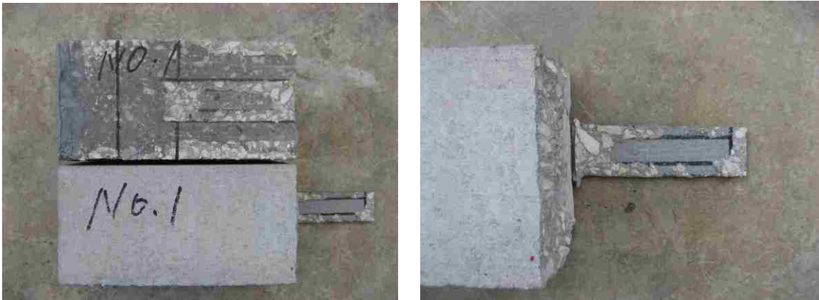
Figure 4.26. The failure mode of a typical conditioned specimen reinforced with galvanized coating steel fibers (RG 1, Failure Mode 3)
