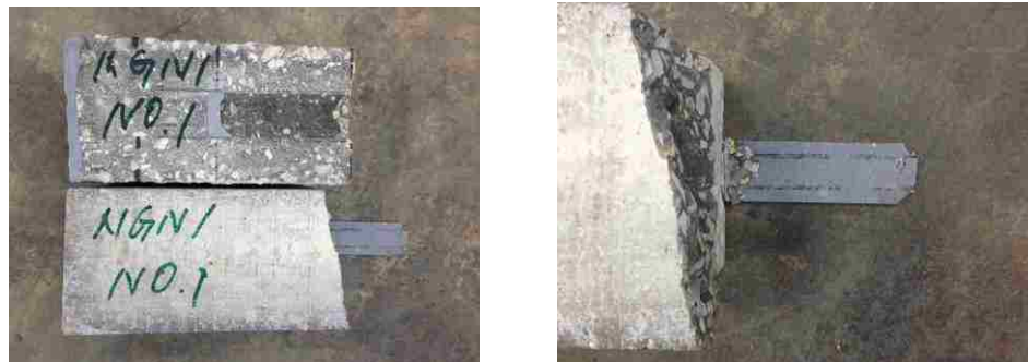
Figure 4.43. A representative failed specimen reinforced with micro-fine brass coating steel fibers under tap water (3,000 hours)
