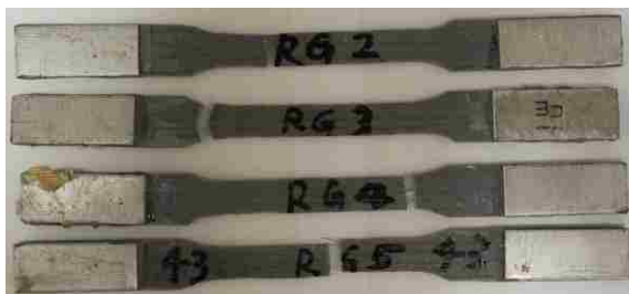
Figure 4.96. Representative tensile failure specimens
