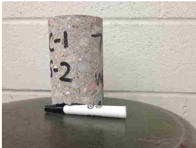
Figure 5.31. The representative concrete cylinder extracted from Southview Bridge
