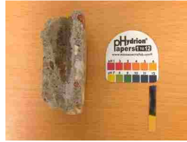
pH measurements at various locations (Southview Bridge)
