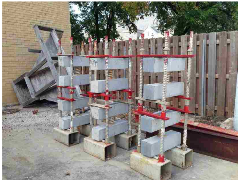
Figure 4.81. Spring-loaded fixture and the testing samples under the real-time exposure
