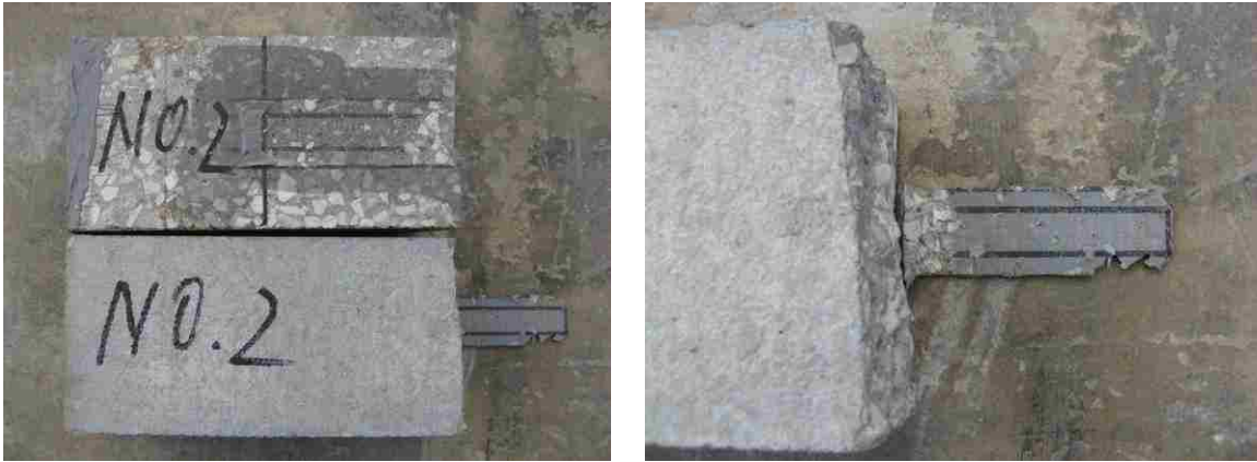
Figure 4.28. The failure mode of a typical conditioned specimen reinforced with brass coating steel fibers (RNG 2, Failure Mode 3)
