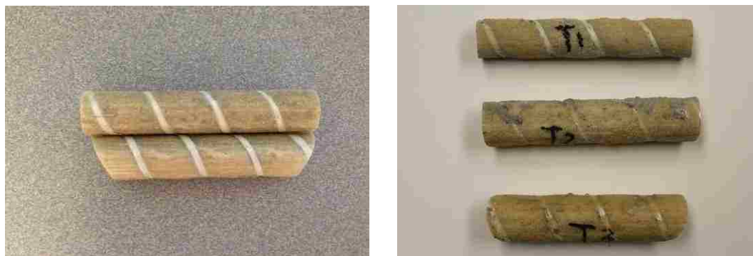
Figure 5.36. The extracted GFRP samples from Southview Bridges (left) and Sierrita de la Cruz Bridge (right)
