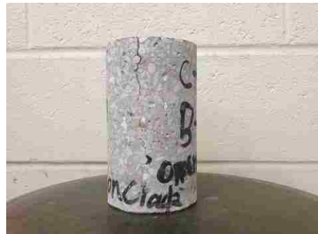
Figure 5.34. A representative concrete core with crack
