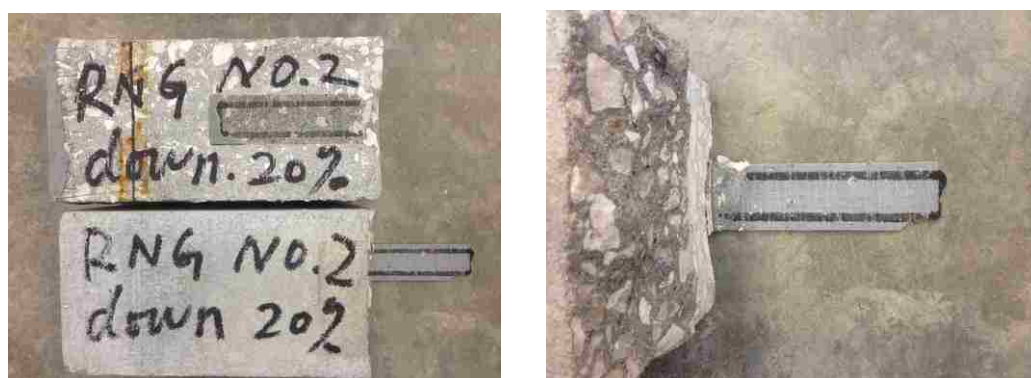
Figure 4.86. A typical failed RNG specimen reinforced (loaded 20%) exposed to field environment
