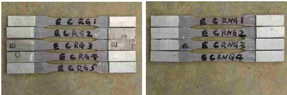
Figure 4.14. The samples with galvanized (left) and brass coating (right) steel fibers
