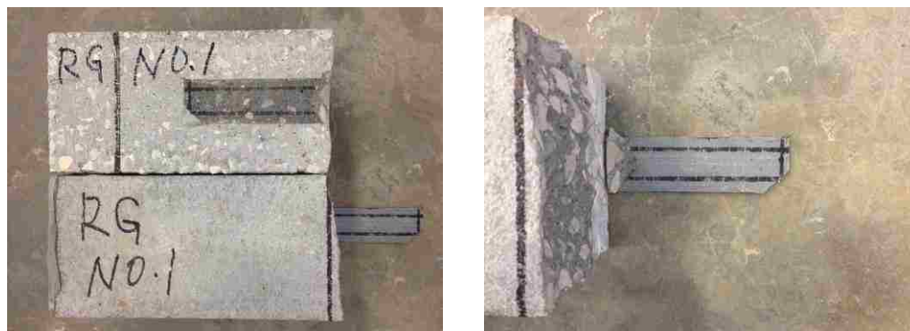
Figure 4.84. A typical failed RG specimen reinforced (unloaded) exposed to field environment
