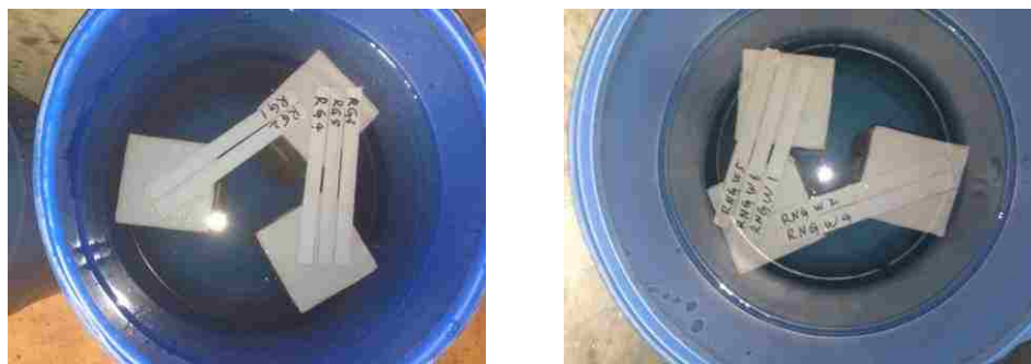
Figure 4.39. SRP specimens in tap water
