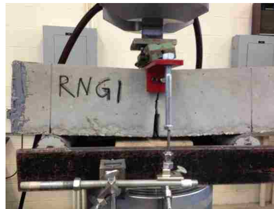
Figure 4.21. A typical failed SRP specimen
