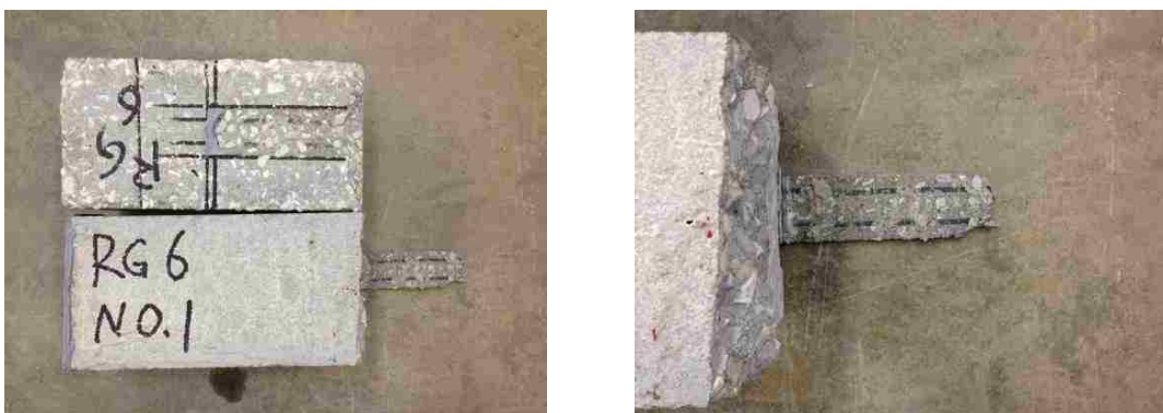
Figure 4.59. Failed control specimen (4,000 hours)
