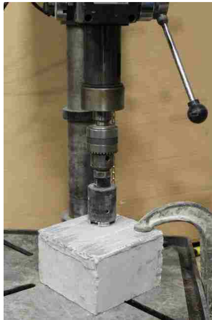
Figure 4.9. The process of drilling core
