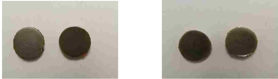
Figure 5.38. Prepared GFRP samples from Southview Bridge (left) and Sierrita de la Cruz Bridge (right) for SEM and EDS
