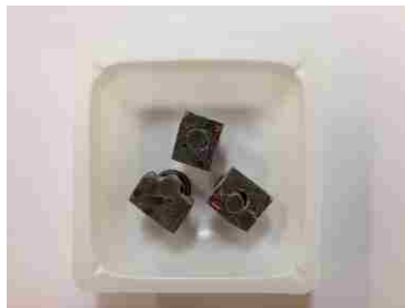
Figure 5.39. Prepared GFRP samples from core C-1 B-3 and core C-2 B-3 of Walker Bridge
