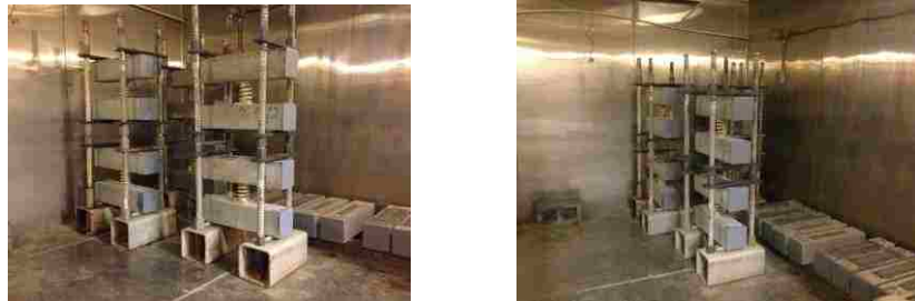
Figure 4.15. Spring-loaded fixture and the testing samples in environmental chamber
