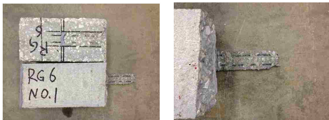
Figure 4.73. A failed control RG specimen (4,000 hours)
