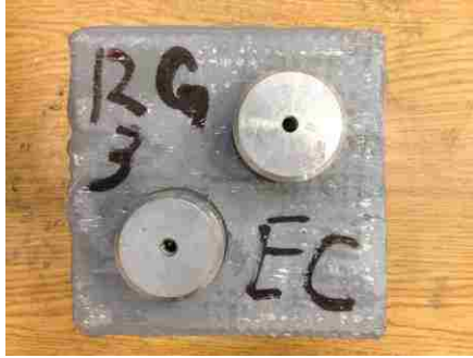
Figure 4.32. A typical adhesion fixture
