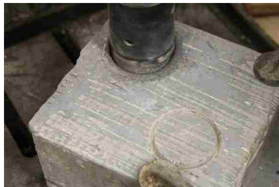
Figure 4.8. The detailed process of drilling core
