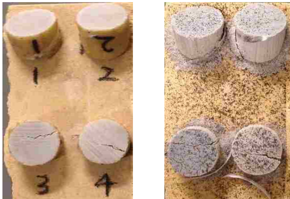
Figure 5.49. The #6 samples of before (left) and after (right) test for Sierrita de la Cruz Bridge
