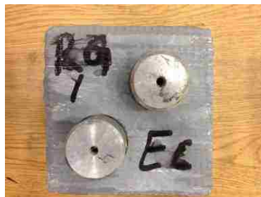
Figure 4.12. A typical pull-off specimen
