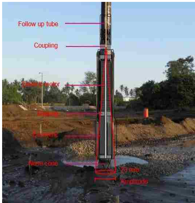
Figure 4.50. V23, Vibratroy probe schematic
