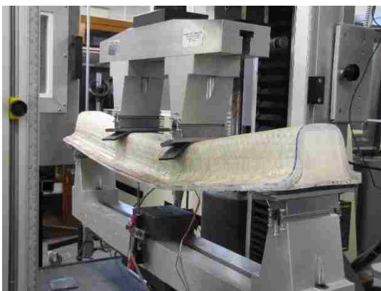
Figure A.10. Four-point flexural tests for Type 3 long beams
