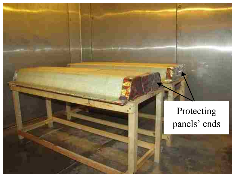
Figure 8. PU sandwich panels within environmental test chamber
