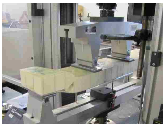
Figure A.9. Four-point flexural tests for Type 2 long beams
