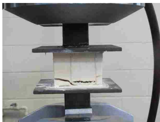
Figure A.4. Flatwise tensile tests for types 1 and 2
