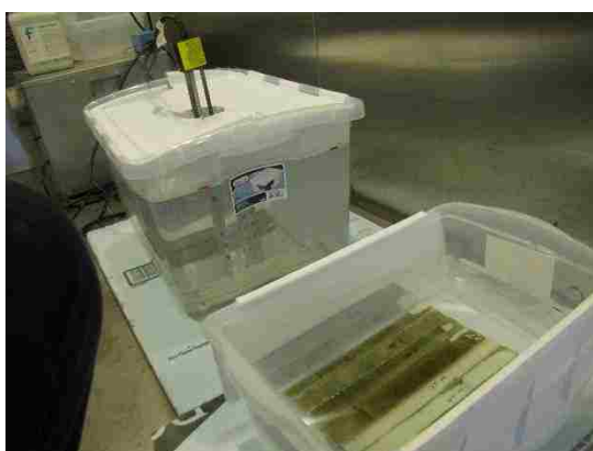
Figure E.2. Deicing solution at room and elevated temperatures
