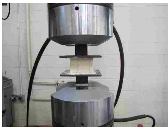
Figure A.4. Flatwise tensile tests for types 1 and 2
