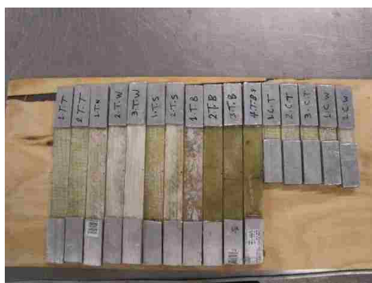
Figure A.1. Material characterization for polyurethane foams and GFRP composites
