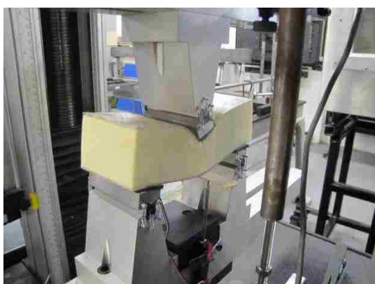
Figure A.5. Three-point flexural tests for Type 1 short beams
