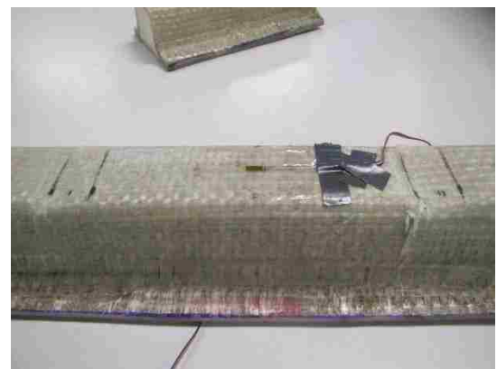
Figure A.10. Four-point flexural tests for Type 3 long beams
