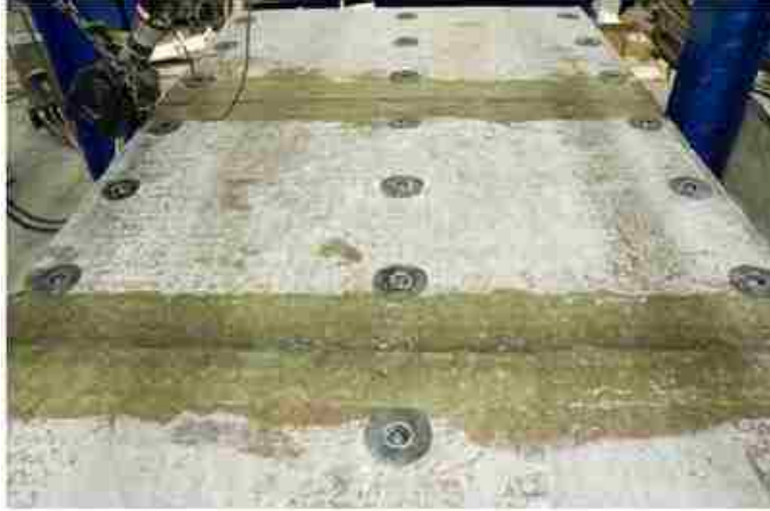
Figure 2.9. Panel-to-girder connection using bolts (Davalos et al. 2012)
