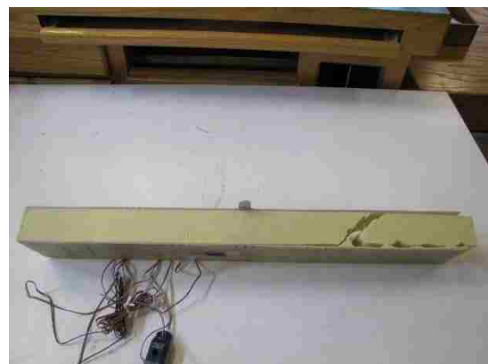
Figure A.8. Four-point flexural tests for Type 1 long beams
