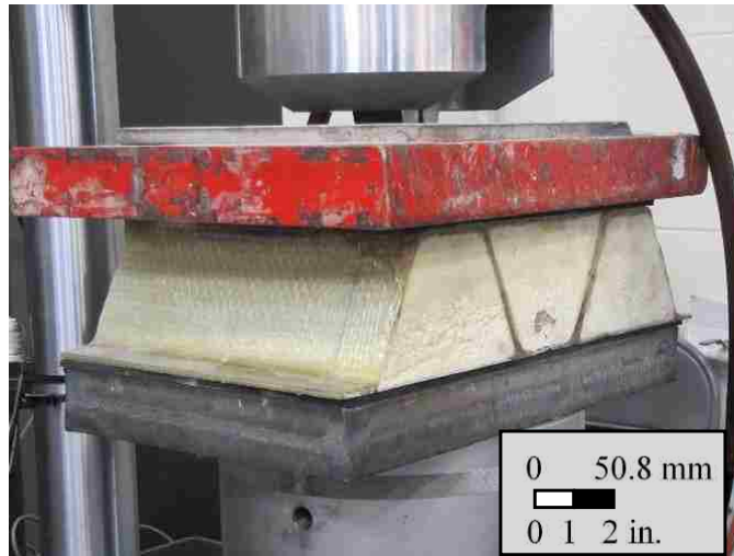
Figure 7. Crushing test setup
