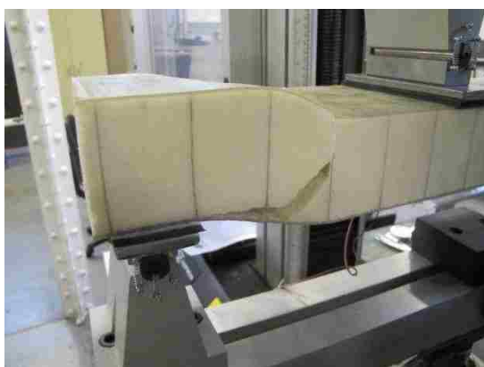
Figure A.9. Four-point flexural tests for Type 2 long beams
