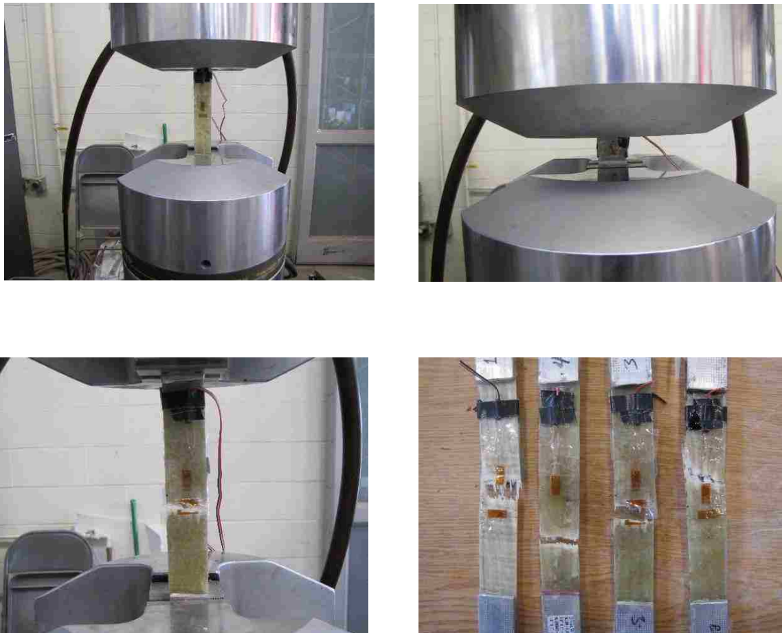
Figure A.2. Material characterization for GFRP composites under compression and tension tests
