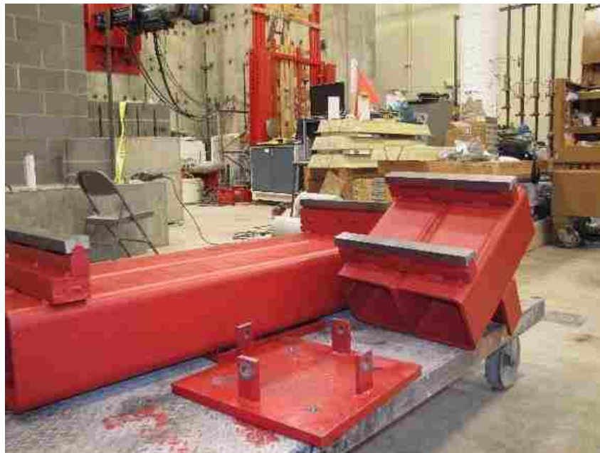
Figure C.1. Fabricated steel test fixture for mid-scale panel testing
