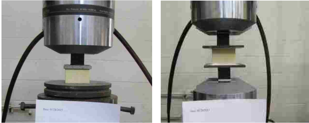
Figure 3. Test setup for flatwise sandwich: (a) compressive test and (b) tensile test for Type 1
