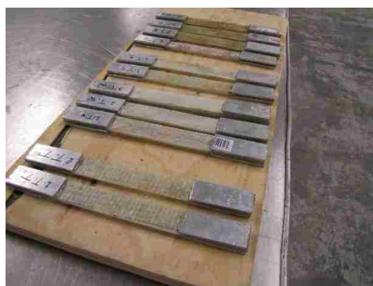
Figure A.1. Material characterization for polyurethane foams and GFRP composites
