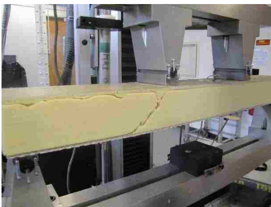
Figure A.8. Four-point flexural tests for Type 1 long beams
