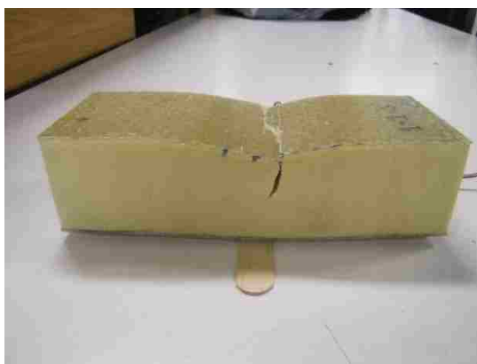
Figure A.5. Three-point flexural tests for Type 1 short beams
