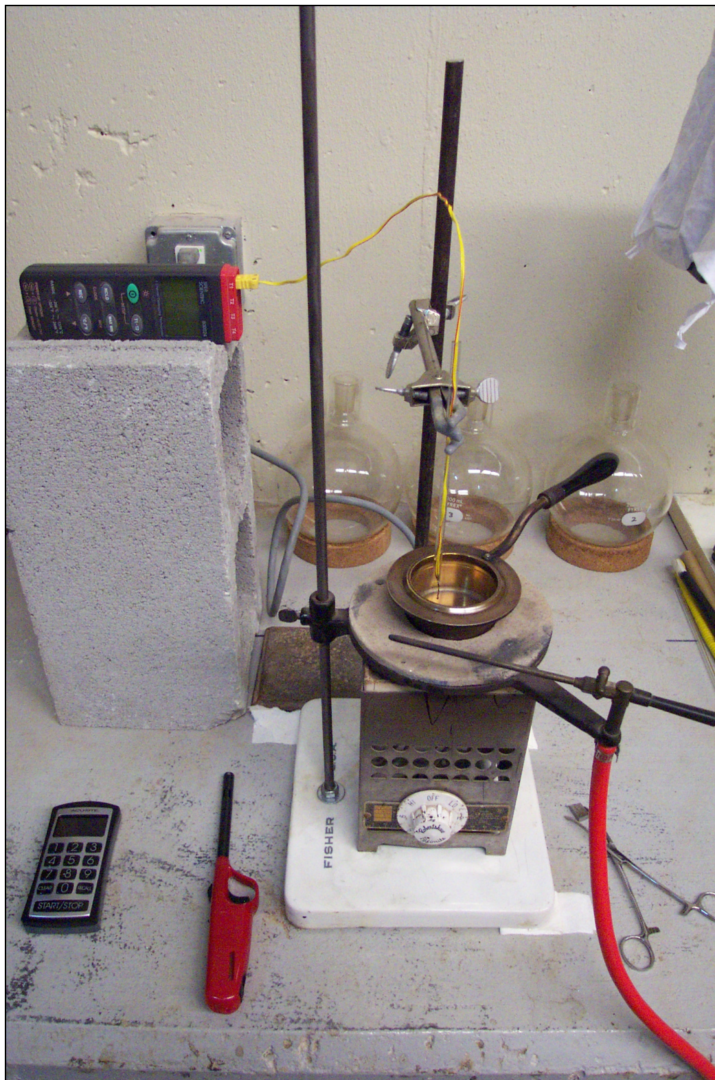
Figure 3.6. Flash Point Test Setup
