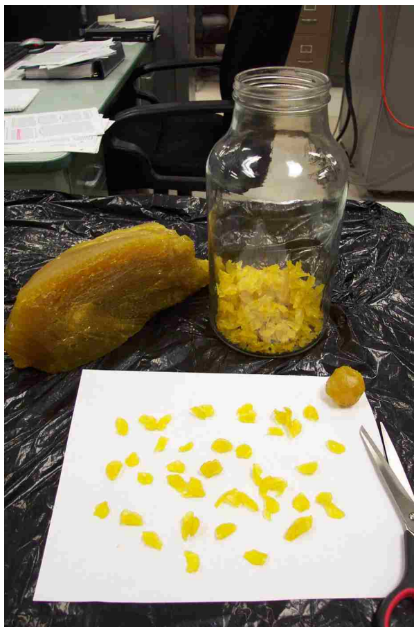
Figure B7. Earliest Method of Rubber Plug Size Reduction
