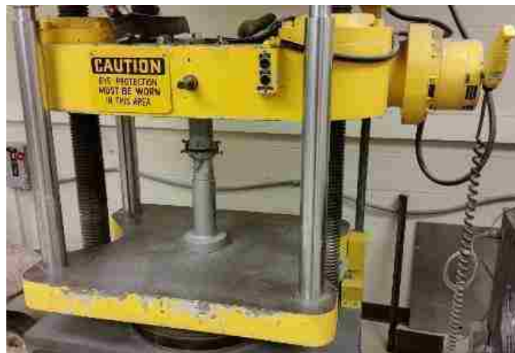
Figure 5.4. UHPC compressive strength setup
