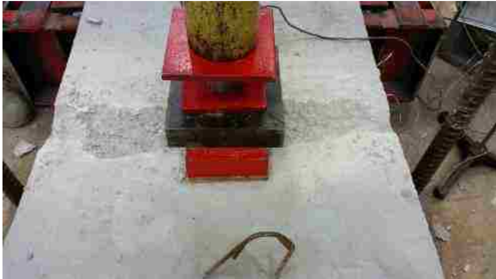
Figure 6.1. Concrete crushed on compression zone on panel FCC3
