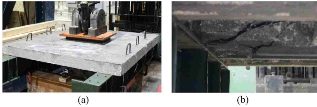
Figure 2.10. Test procedure (a) test setup; (b) failure mode (Ghasemi et al., 2016)
