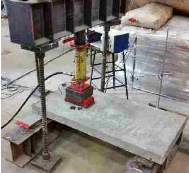
Figure 6.43. Panel SUN3 test setup
