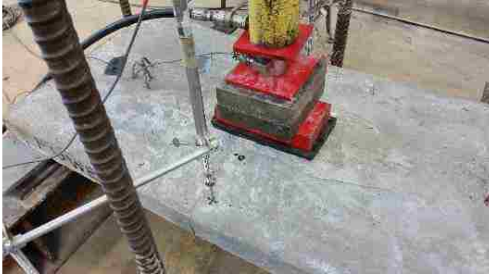
Figure 6.9. Panel FUC3 after failure
