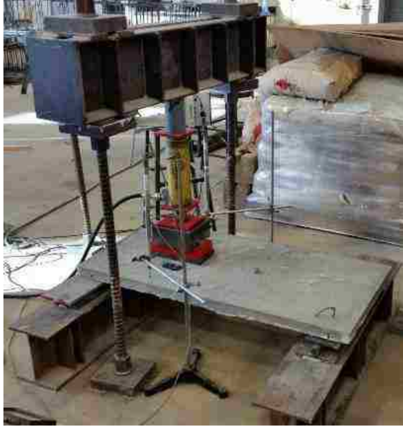
Figure 6.54. Panel SUN2 test setup
