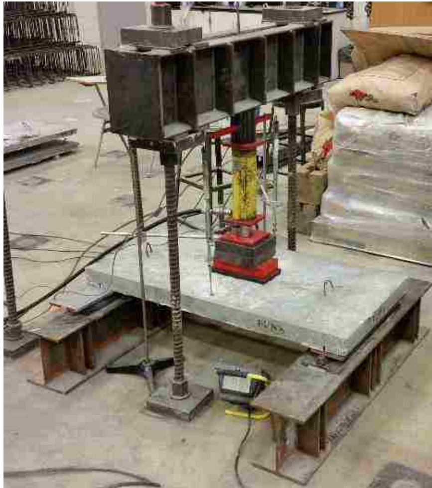
Figure 6.19. Panel FUN3 test setup
