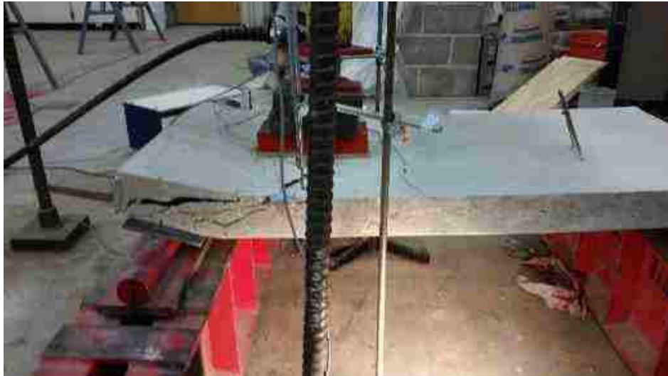
Figure 6.35. Diagonal tension failure on panel SCC3
