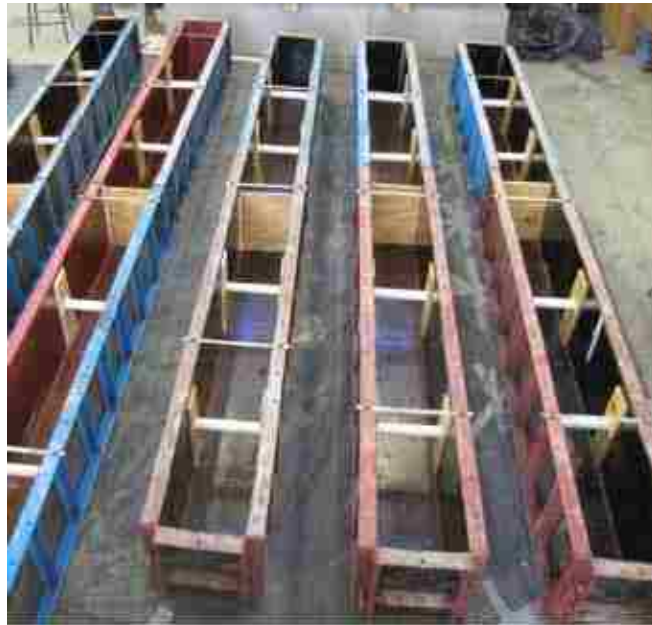
Figure 3.1 Concrete beams cast using the parent concrete for RCA production in laboratory
