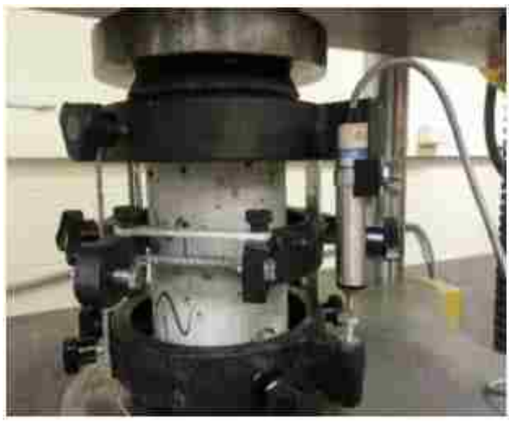
Figure 5.2 Modulus of elasticity test setup
