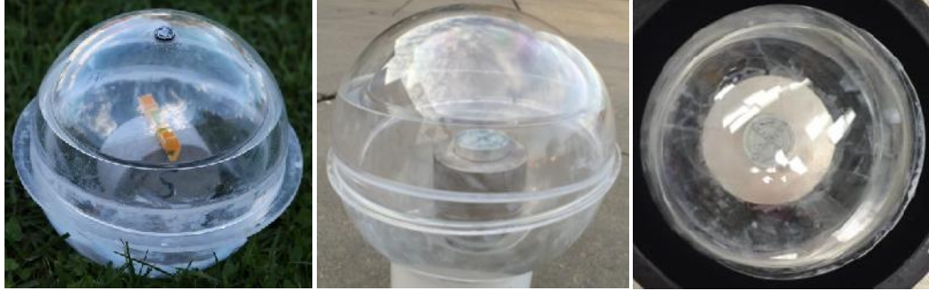
Figure 2.9. Prototype: (a) APSS with one N42 magnet, (b) APUS with two stacked N42 magnets, and (c) APUS with one N45 magnet.
