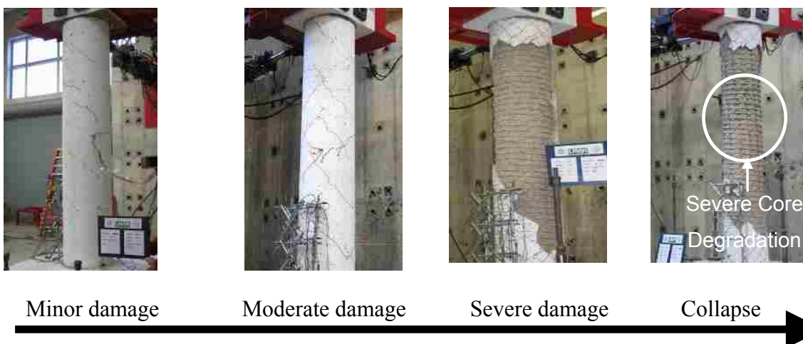
Figure 6.11 Categorization of Damage States under Pure Torsion
