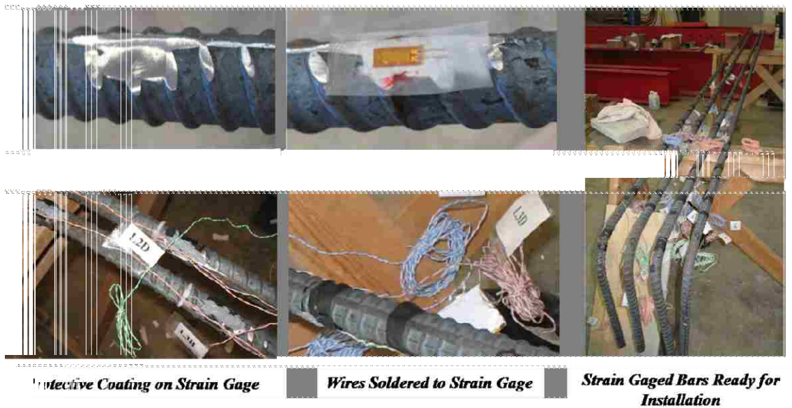
Figure 3.7 Applying Strain Gages on Longitudinal Reinforcement
