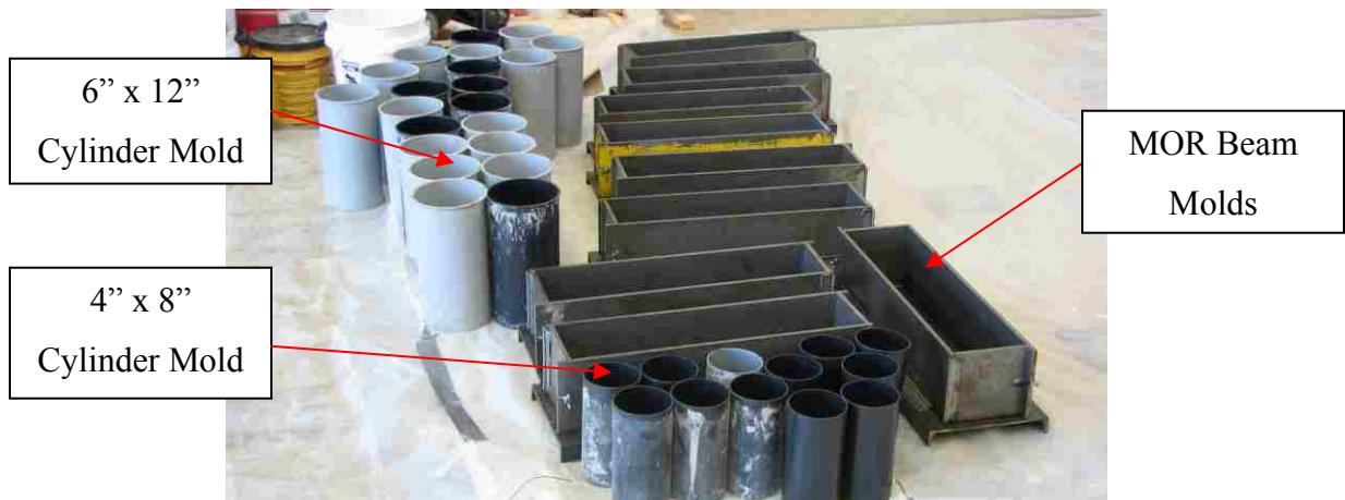
Figure 3.20 Auxiliary Specimens for Concrete Material Testing
