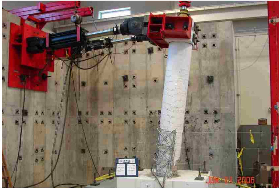
Figure 3.4 Photo of the Test Setup for Column under Flexure
