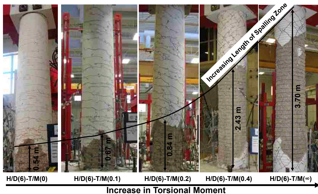
Figure 4.50 Effect of Combined Loading including Torsion on Spalling Distribution
