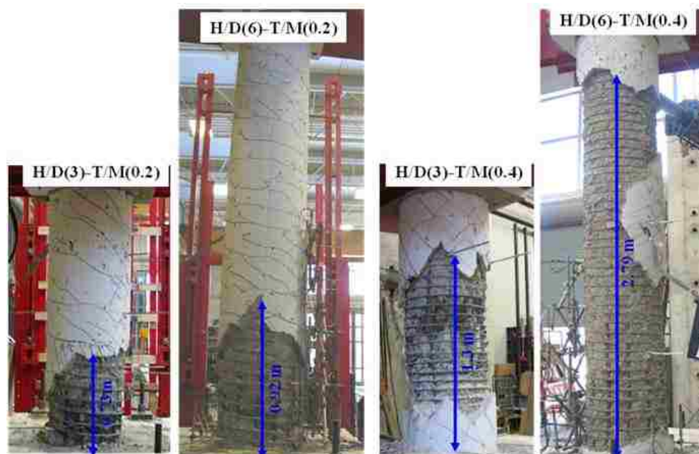
Figure 4.60 Effect of Shear Span on Damage Distribution under Combined Bending and Torsional Moments
