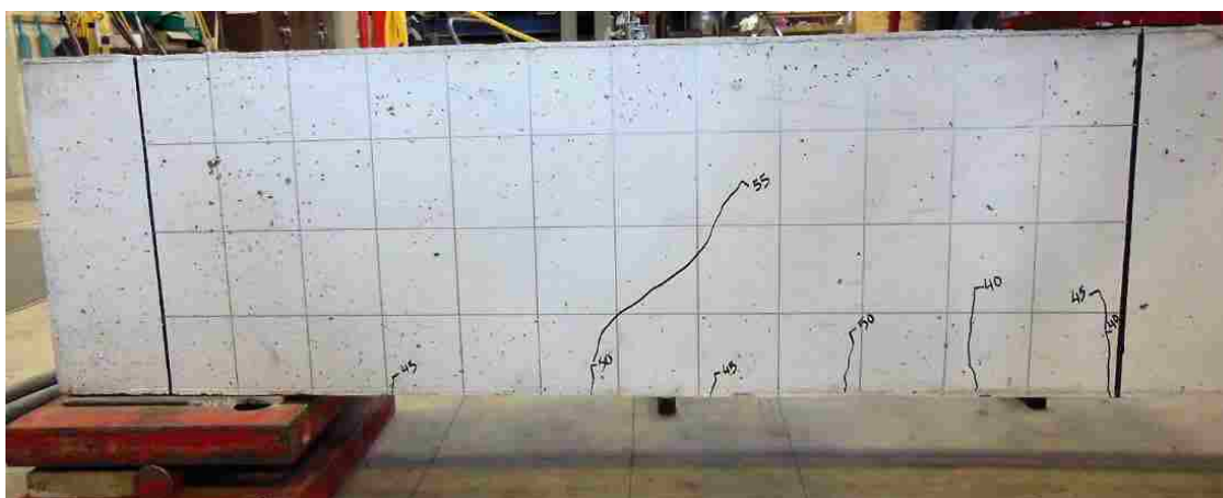
Figure B-8. Cracking Shear in Specimen 60-5N
