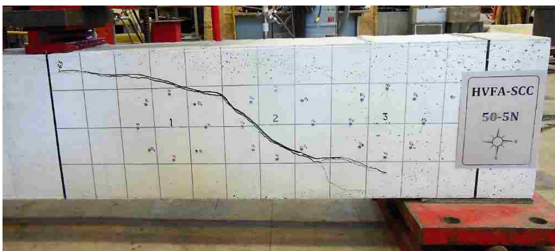
Figure B-2. Ultimate Shear in Specimen 50-5N
