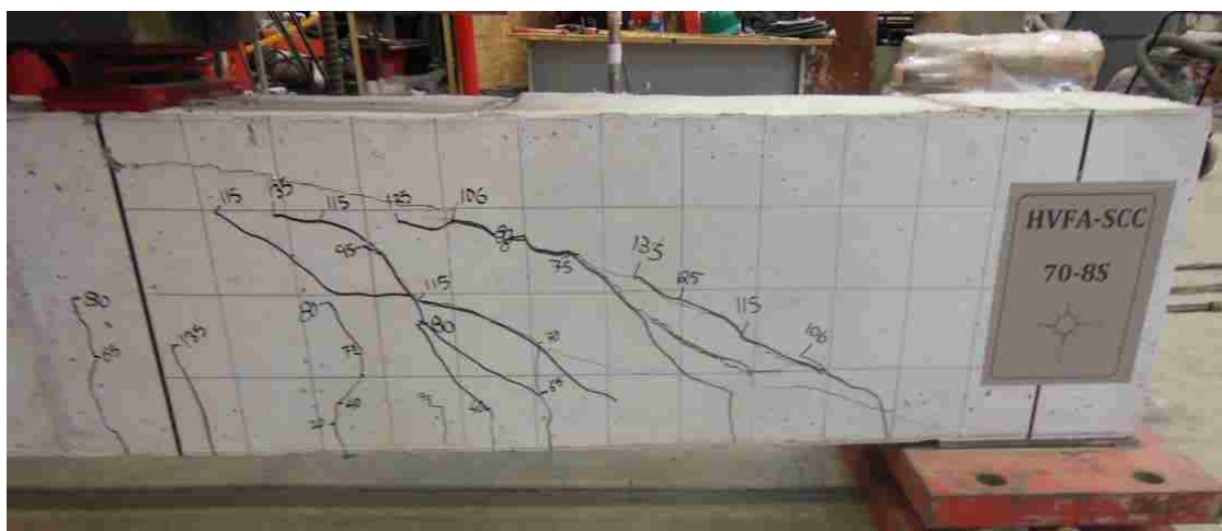
Figure B-23. Ultimate Shear in Specimen 70-8S
