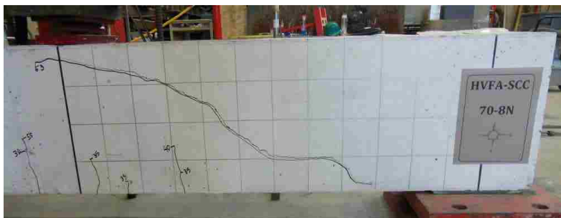
Figure B-20. Cracking Shear in Specimen 70-8N
