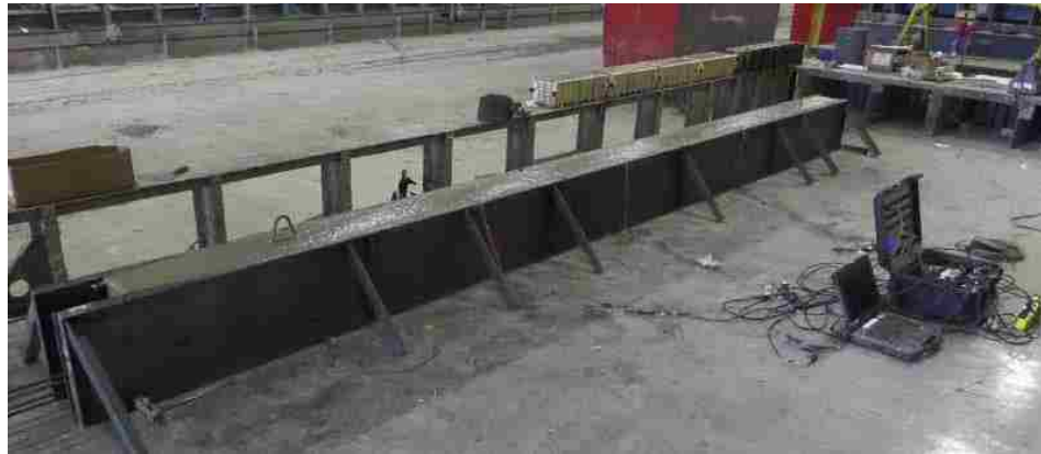
Figure F-3. DAS Collecting Data at Precast Plant
