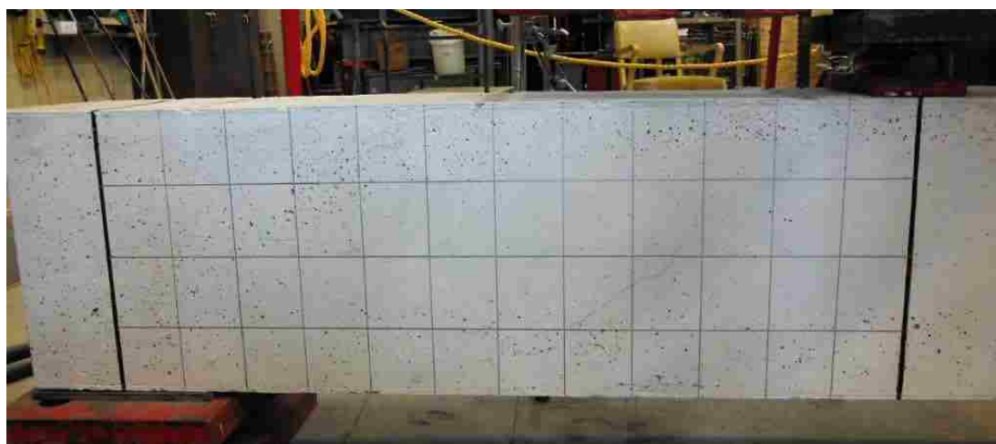
Figure B-1. Cracking Shear in Specimen 50-5N
