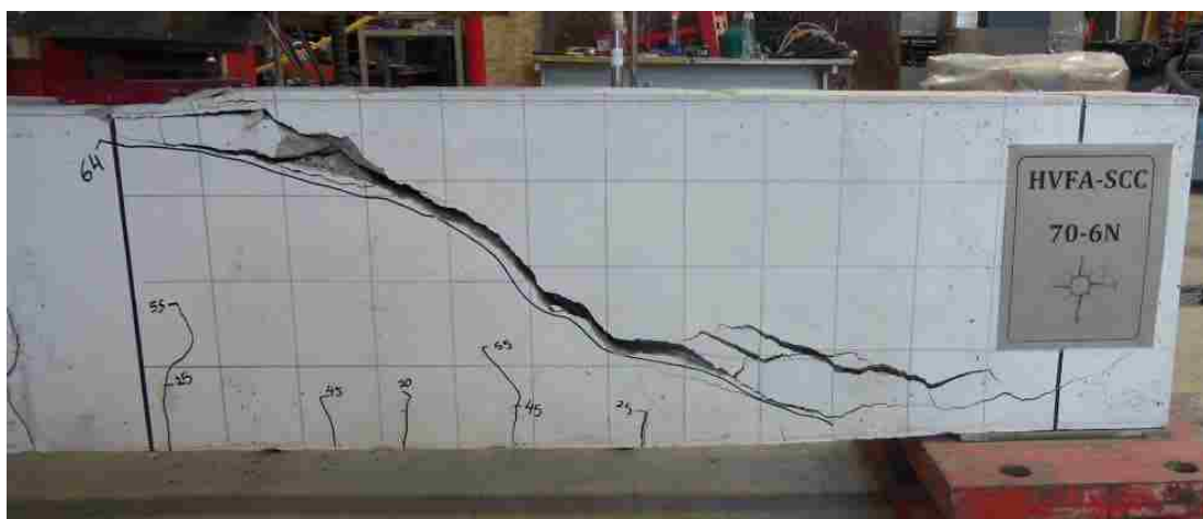
Figure B-19. Ultimate Shear in Specimen 70-6N
