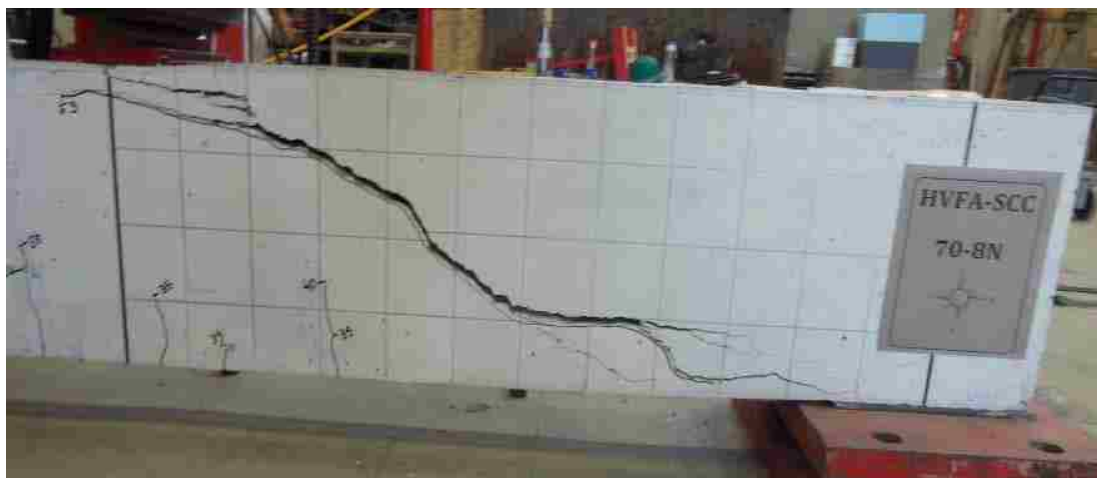
Figure B-21. Ultimate Shear in Specimen 70-8N
