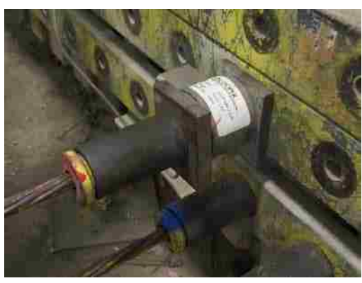
Figure F-2. Load Cell Installation Detail
