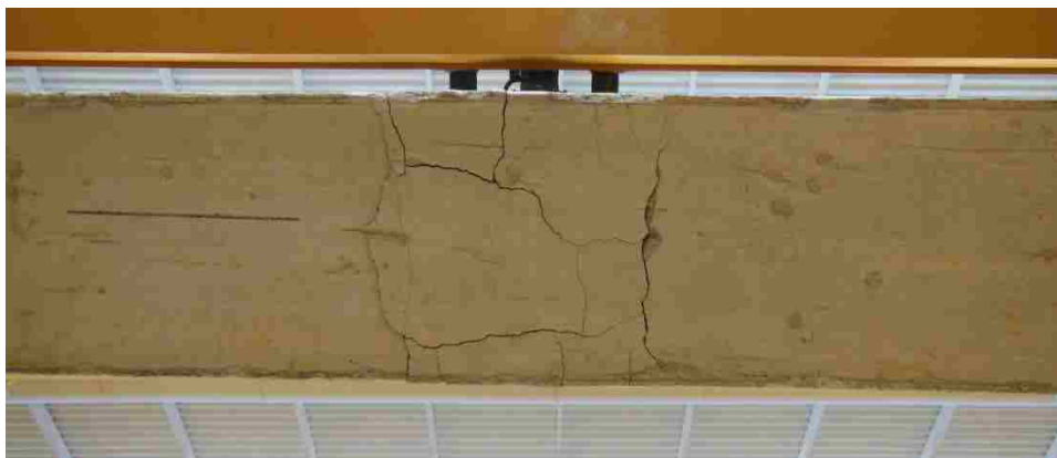
Figure D-4. Crack Pattern of Specimen BWOC-50 (Bottom View)
