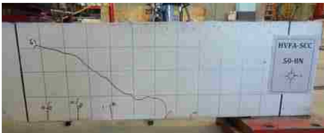
Figure B-5. Cracking Shear in Specimen 50-8N
