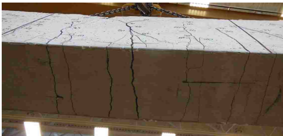
Figure D-18. Crack Pattern of Specimen REF-70 (Bottom View)
