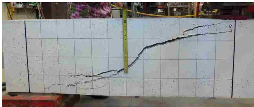
Figure B-4. Ultimate Shear in Specimen 50-6N
