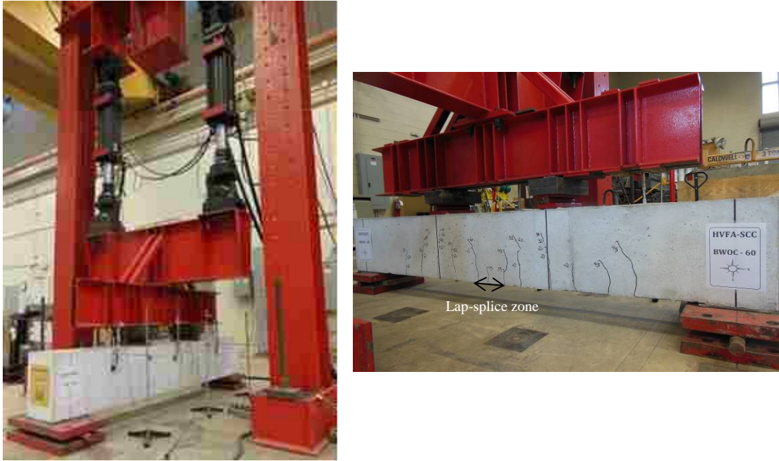
Figure 2. Test setup, instrumentation, and testing and failure mode of a beam specimen.
