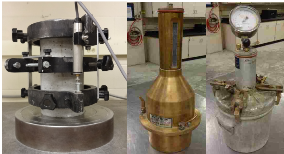
Figure 3.5 Modulus of Elasticity Yoke, Brass Volumetric Meter, and Pressure Meter (from left to right)
