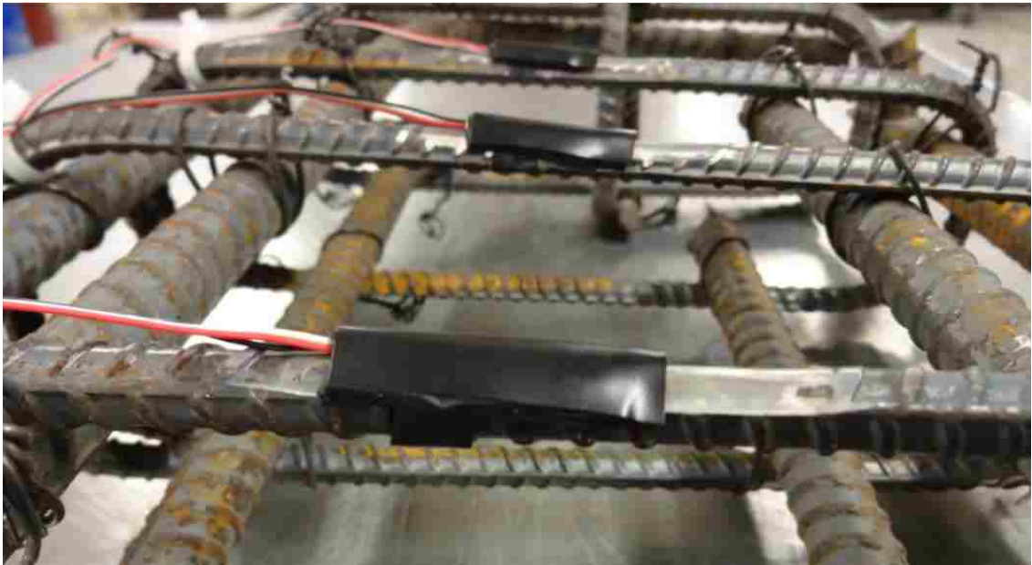
Figure 3.19 Strain Gages Attached to Shear Reinforcement
