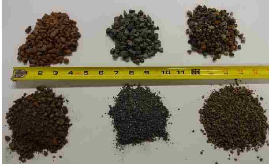
Figure 3.2 From Left to Right: Expanded Shale, Expanded Slate, Expanded Clay. Coarse Aggregates Top Row, Fine Aggregates Bottom Row
