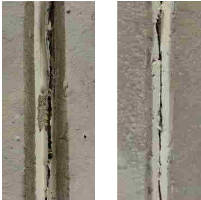
Figure 4.1 Typical Shear Plane Crack Normalweight Concrete Monolithic Interface (left), Shale Sand-lightweight Concrete Monolithic Interface (right)
