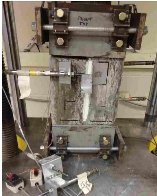
Figure 3.41 Detached DC-LVDTs on specimen S-CL-CJ-R-1
