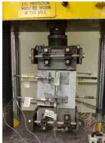
Figure 3.14 Typical Support Conditions for Testing
