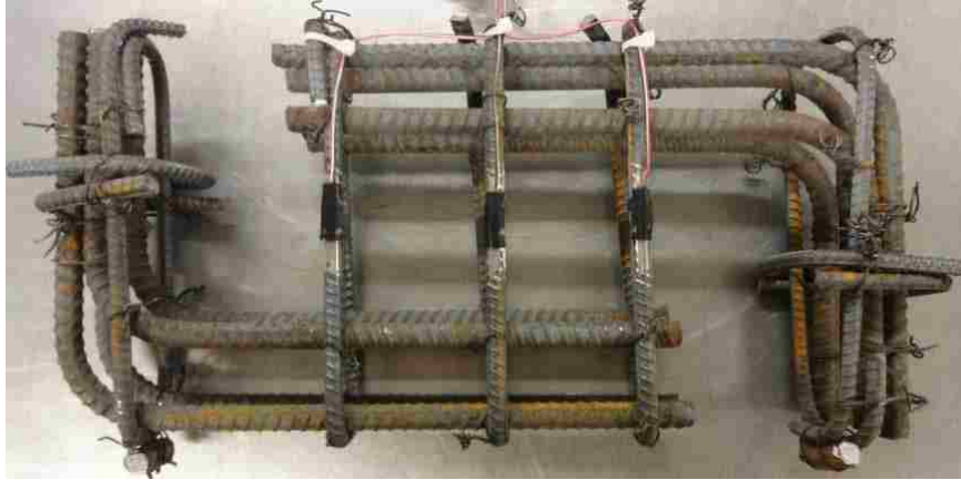
Figure 3.9 Reinforcement Cage with Strain Gages
