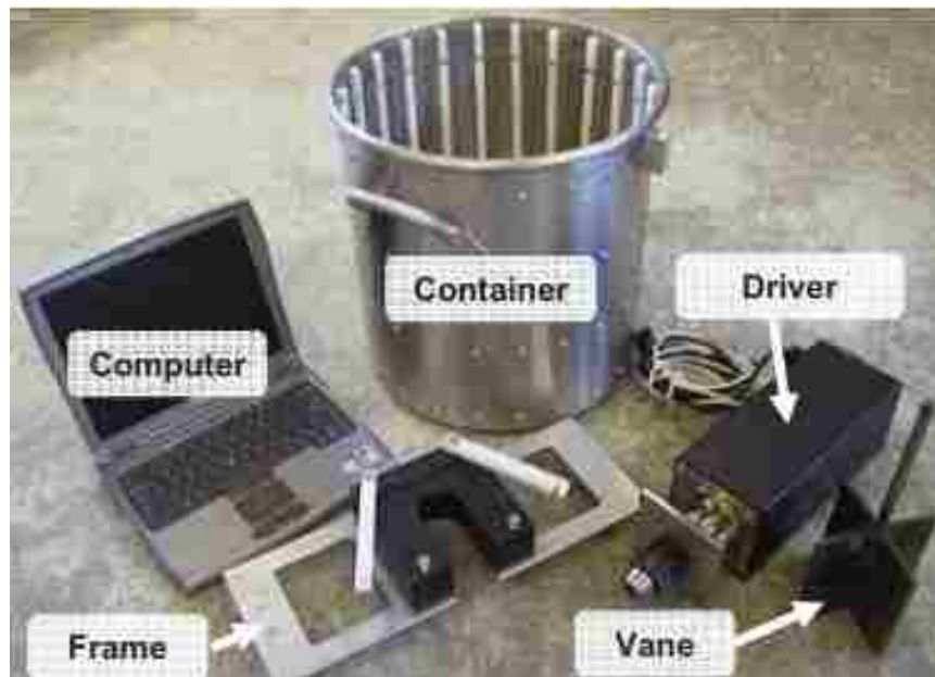
Figure 3-3 ICAR rheometer parts.
