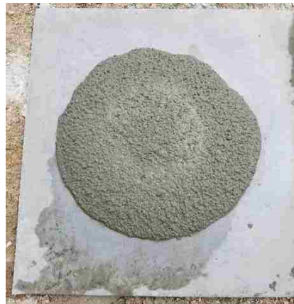
Figure 4-6 Slump flow example.
