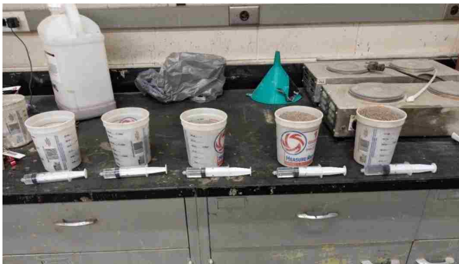
Figure 4-13 Batched weights of the sand and equivalent water to bring the sand to SSD condition.
