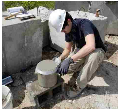
Figure 4-7 Air content test.
