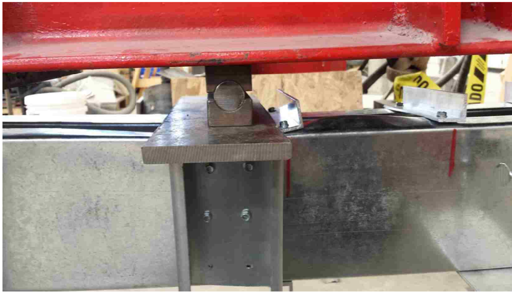
Figure 4.2 Typical Failure of Crimp in Tension Flange
