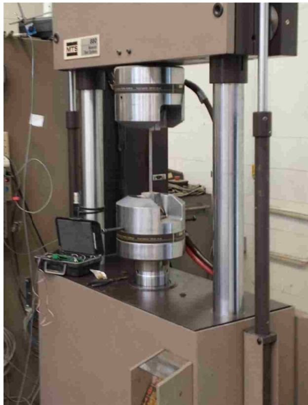
Figure 3.1 Typical Tensile Coupon Test Setup
