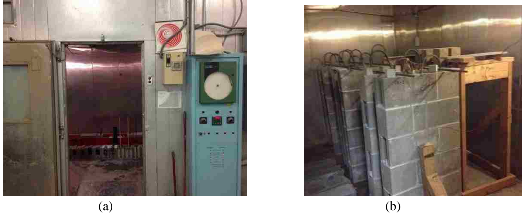
Figure 7. Specimens in environmental chamber (a) strengthened masonry units, (b) strengthened RM walls
