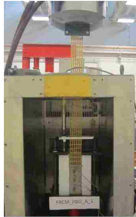
Heating and cooling chamber
