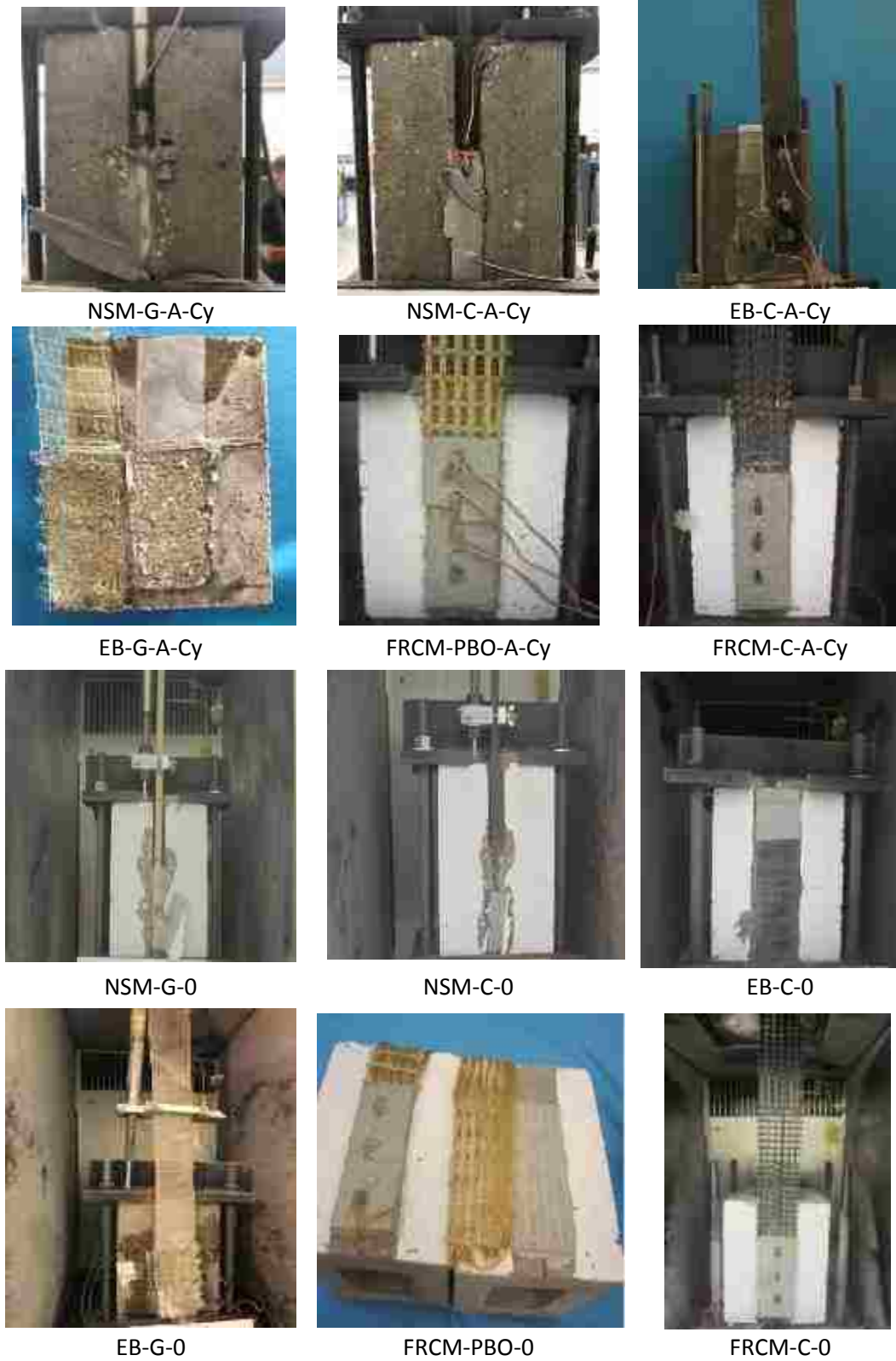
Figure10. Modes of failure for all strengthening system in different temperatures
