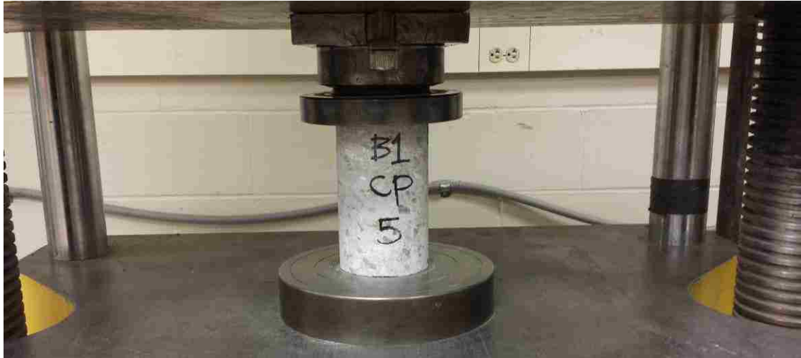
Figure 5.19 Compressive strength test setup of cores.
