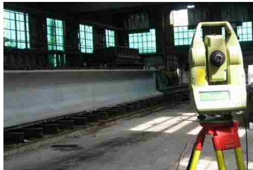
(a) Total station
