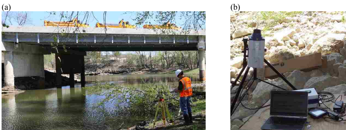
Figure 3. Non-contact remote data acquisition systems. (a) Automated total station; (b) remote sensing vibrometer (RSV-150).
