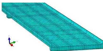
Figure 13. Bridge A7957' FEM geometry.
