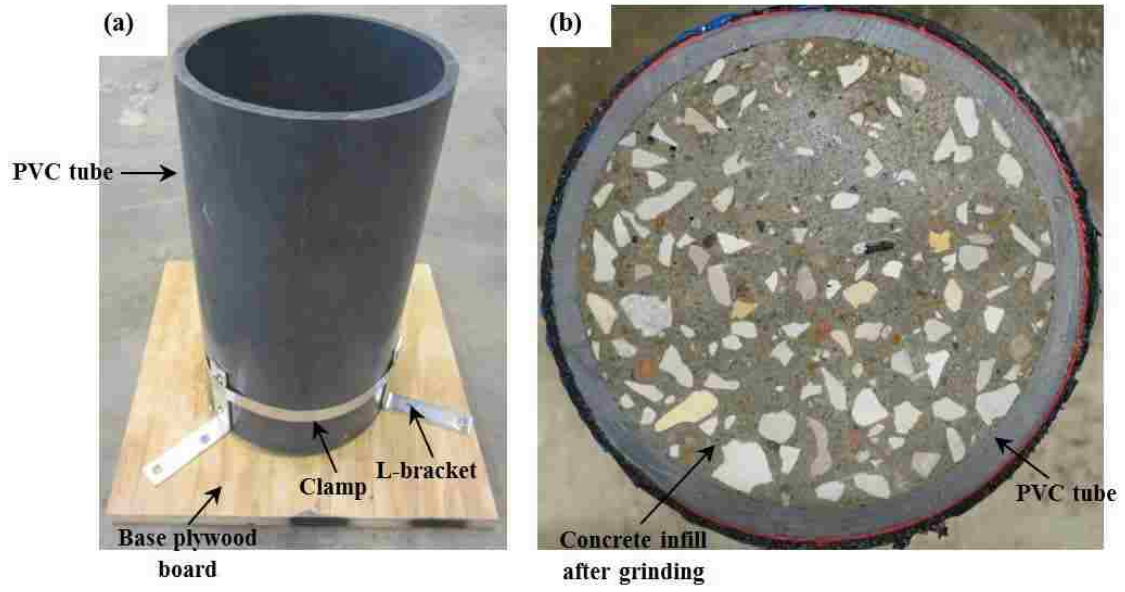
Fig. 1. Preparation of cylinder specimens: (a) PVC tube prior to casting; (b) ground end.
