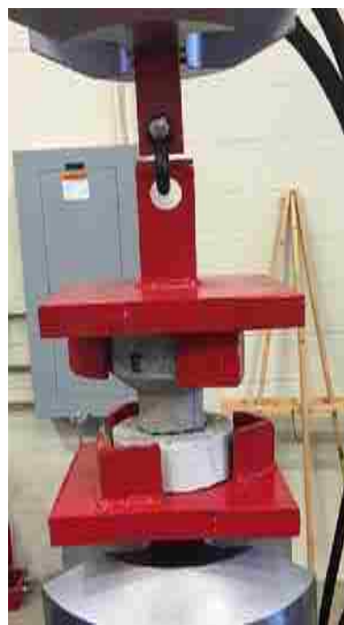
Figure 6-15 Illustration of test set-up for UHPC debonding test
