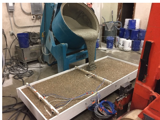
Figure 6-6 Preparation and casting process of UHPC overlay
