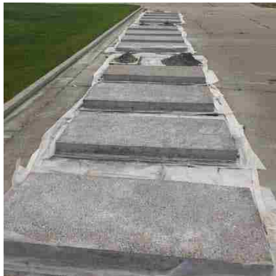
Figure 6-1 Concrete pavement sections as substrate
