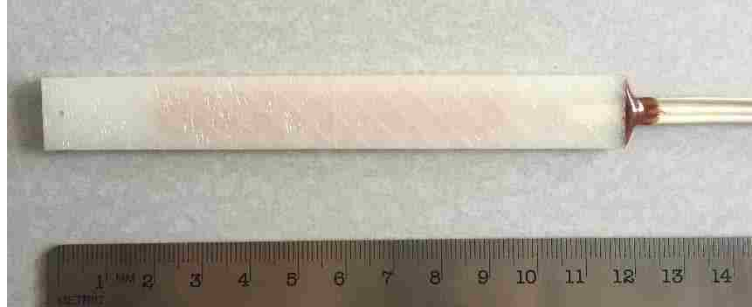
Figure 6-3 Embedded strain gauge for monitoring shrinkage deformation
