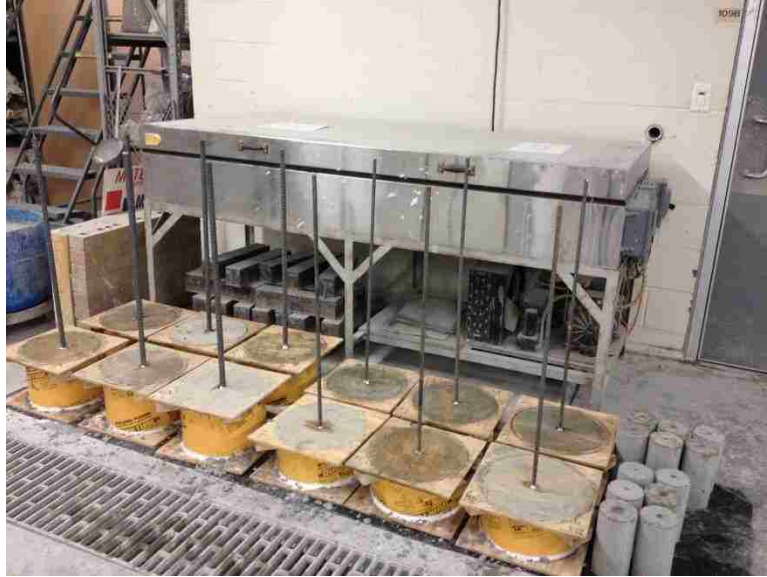
Figure 4.4 Completed Direct Pull-Out Specimens in Molds
