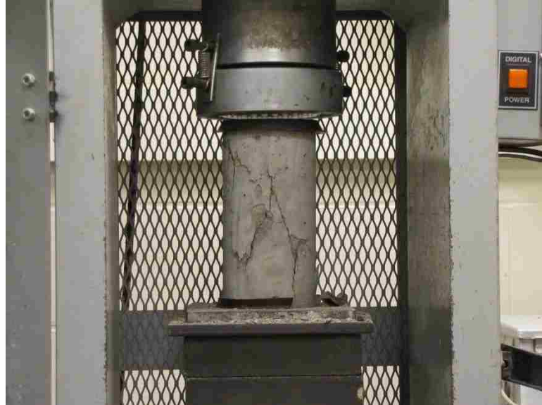
Figure 3.1 Compressive Strength Test
