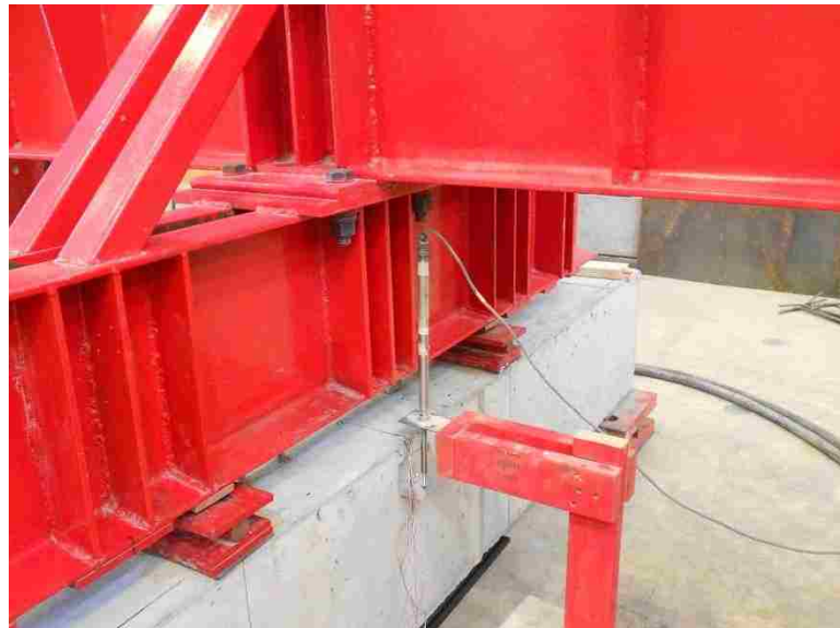
Figure 4.15 LVDT Set-Up for Beam Splice Test
