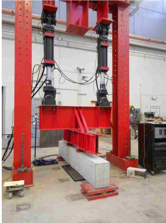
Figure 4.14 Beam Splice Specimens in Testing Load Frame
