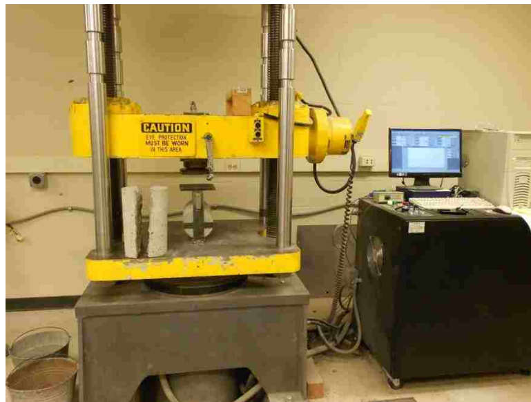
Figure 3.2 Splitting Tensile Failure Mode
