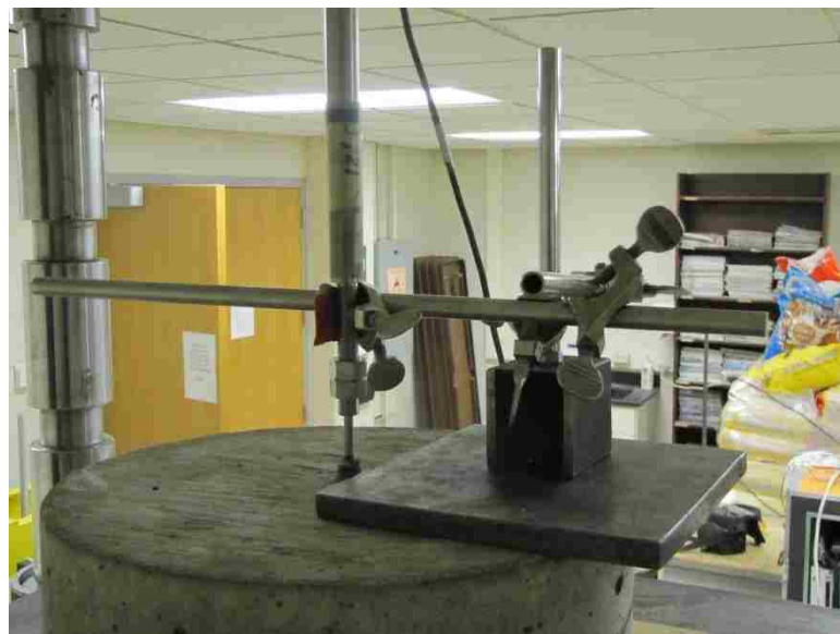
Figure 4.6 LVDT Set-Up for Direct Pull-Out Specimen
