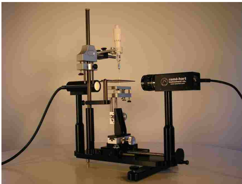
Figure 3.5 Rame-hart goniometer (Wikipedia, 2014)
