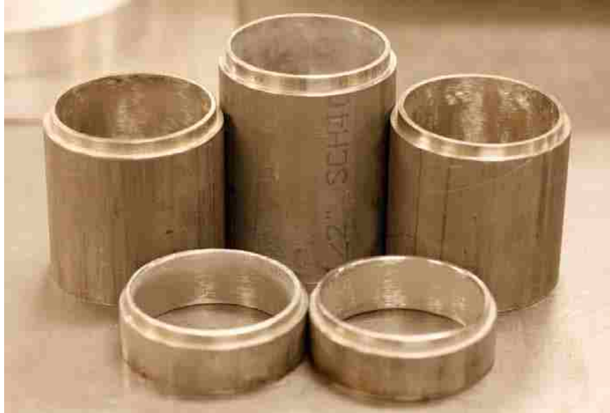
Figure 4.2 stainless steel sample preparation tube
