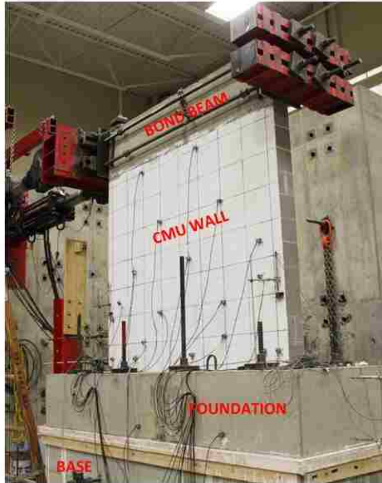
Figure 4.1. Masonry shear wall setup showing components
