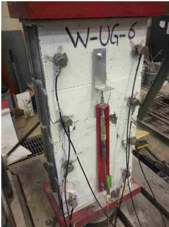
(a) 37% Rubber CMU UngROUTed
