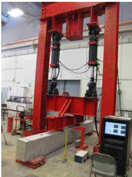
c) Splice test setup with specimen loaded
