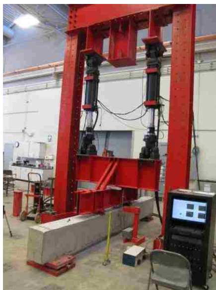
c) Splice test setup with specimen loaded
