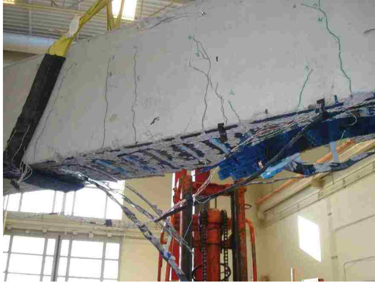
Figure 4.51. Failure of Beam 6
