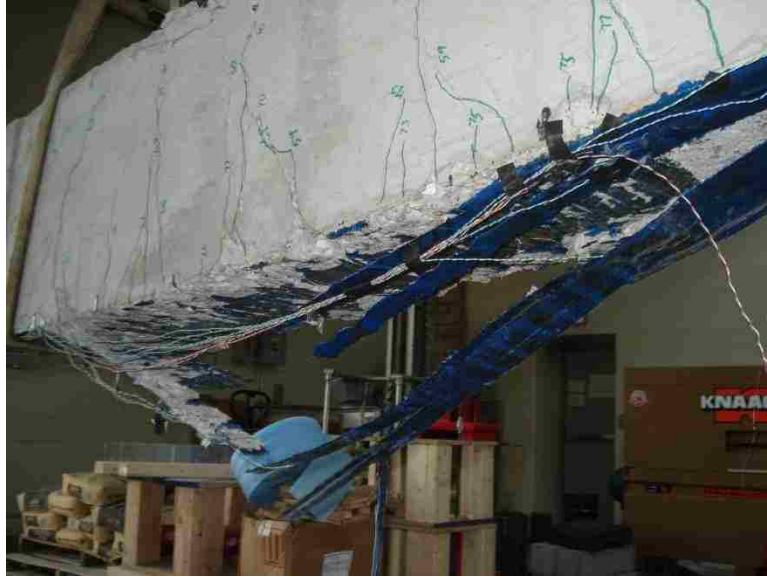
Figure 4.18. Failure of Beam 3
