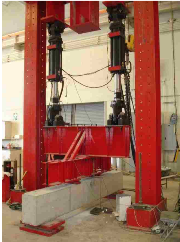
Figure 4.6. Beam Test Setup
