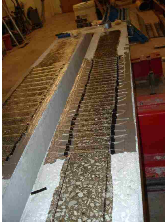
Figure 4.8. During FRP Application
