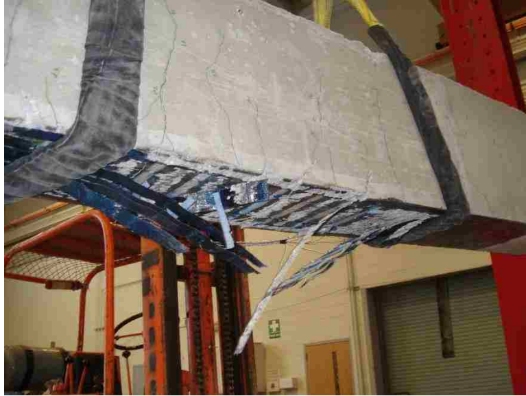
Figure 4.61. Failure of Beam 9
