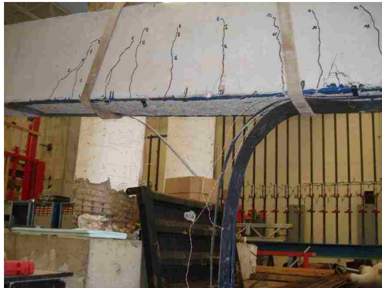
Figure 4.37. Failure of Beam 3
