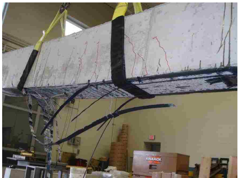
Figure 4.67. Failure of Beam 10
