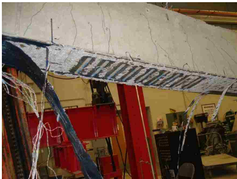
Figure 4.56. Failure of Beam 7
