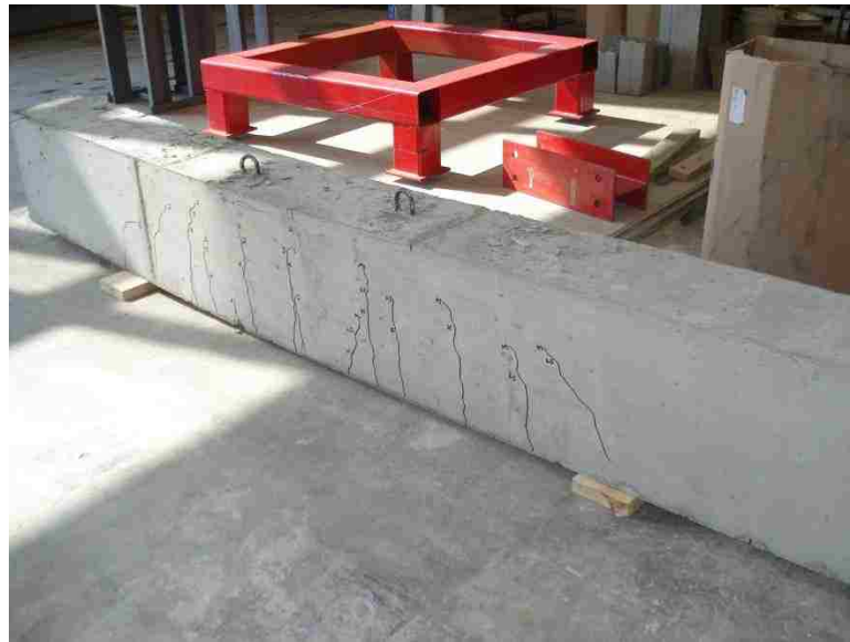
Figure 4.31. Failure of Beam 1
