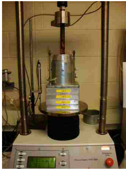
Figure 4.3. Static Undercompaction of Specimens
