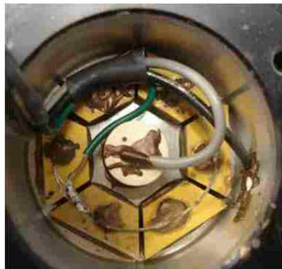
Figure 4.12. Piezoelectric Crystals Mounted in Specimen End Platens
