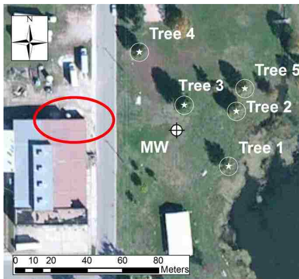
Figure 2. Plan view of the field site showing the five sampled trees. The red ellipse denotes the likely source area. Groundwater flow is towards the park to the east.
