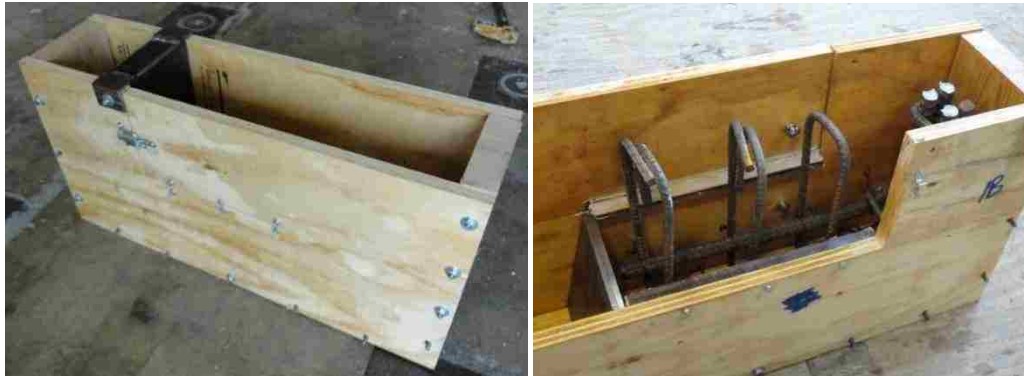
Figure 3.8. Test specimen formwork
