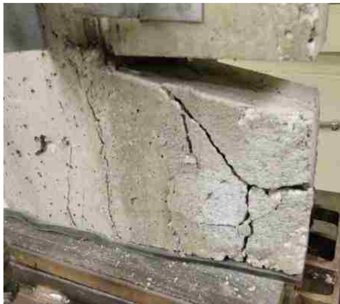
Figure 3.12. Premature flange failure
