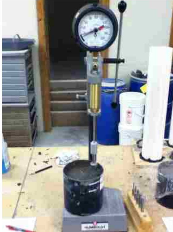
Figure 3.5. Concrete Time of Set Setup
