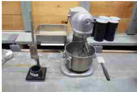
Figure 3.13. Vicat Apparatus and Mixing Equipment
