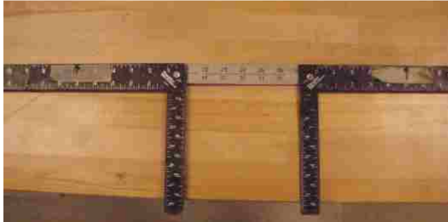
Figure 3.6. Beam Alignment Jig
