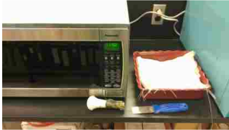
Figure 3.4. Microwave Water Content Station
