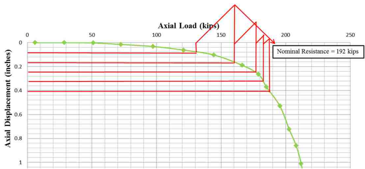
Figure 5.14 Interpretation of A7956 Nom. Resistance Using the Mazerkiewicz (1980) Method
