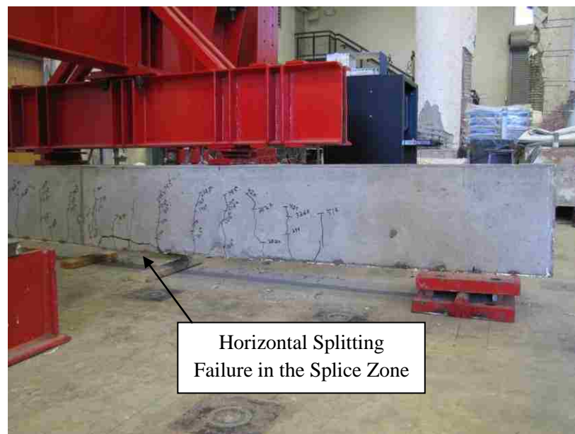
Figure 5.10 – Failed splice specimen
