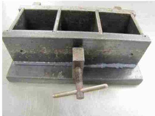
Figure 3.3 – Caulked cube molds
