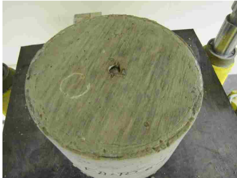
Figure 4.7 – Failed pull-out specimen
