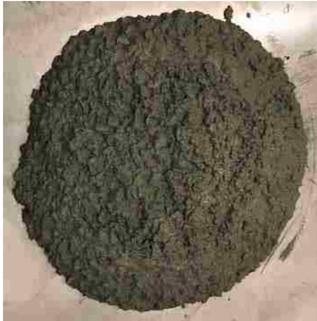
Figure 3.12 Typical slump flow
