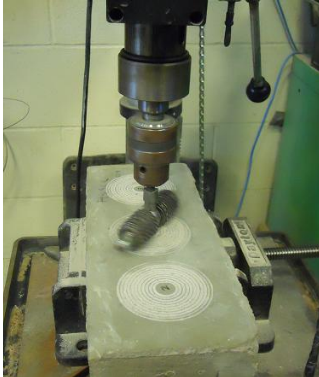
Figure 3.13 - Abrasion Resistance Test In Progress
