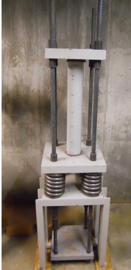
Figure 3.9 - Creep Loading Frame with Specimen
