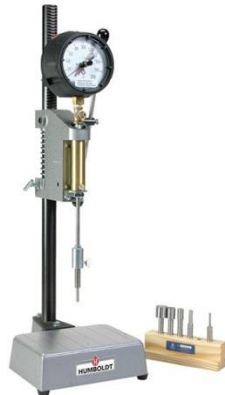
Figure 4.5. Apparatus of Penetration Resistance Test
