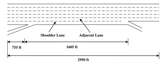
(b) Uncongested data collected site with Six Main Lanes, an On-Ramp and an Off-Ramp
