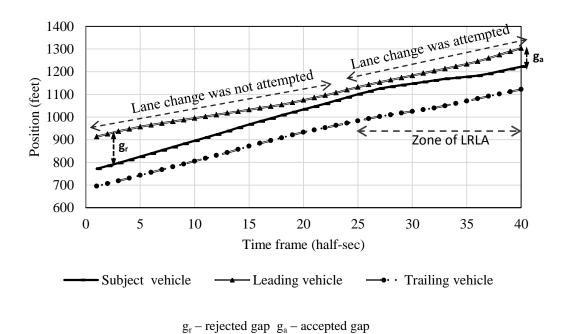
Figure 3 Trajectory of a driver: Need for LRLA
