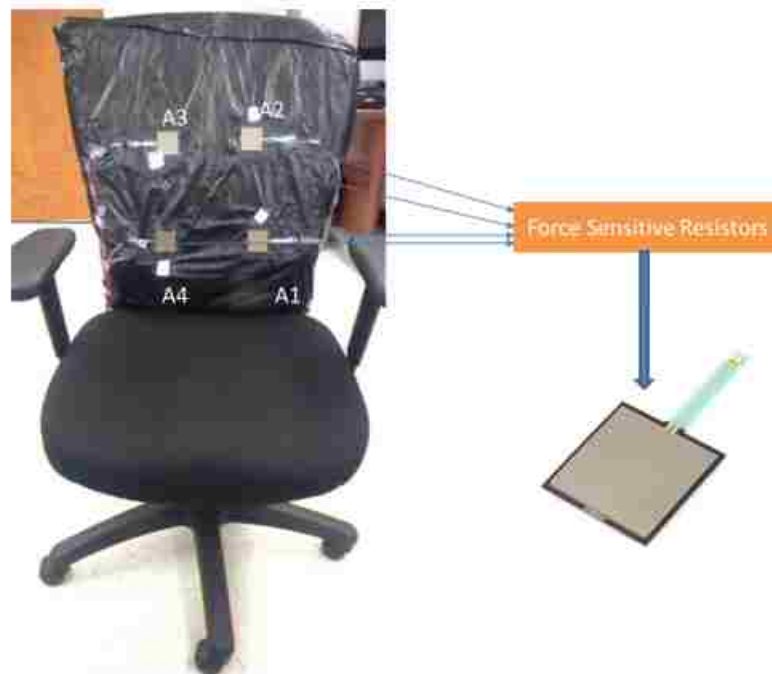
Figure 3.1. Care-Chair Force Sensitive Resistor placement on the backrest of chair
