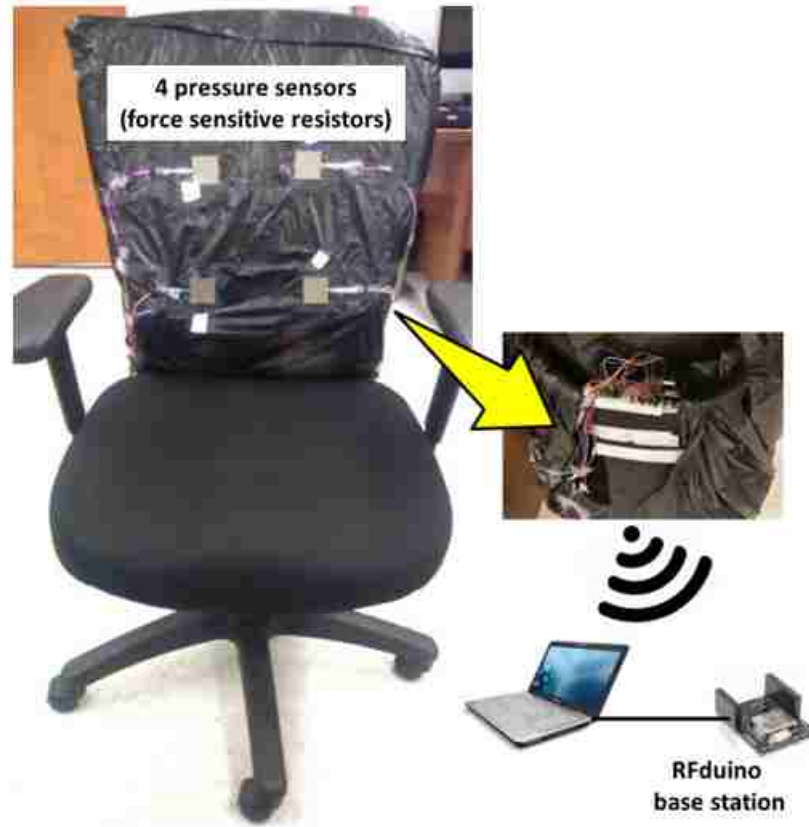
Figure 3.5. Overall Care-Chair system design
