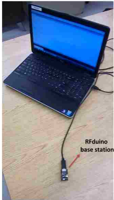
Figure 3.4. RFduino device connected to computer for receiving data from the slave RFduino in the chair
