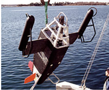
Figure 2.2. Video Plankton Recorder
