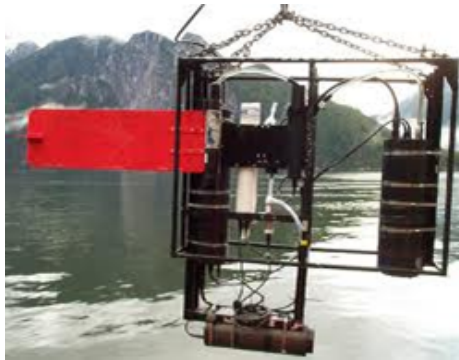
Figure 2.4. ZOOVIS Zooplankton Imaging System
