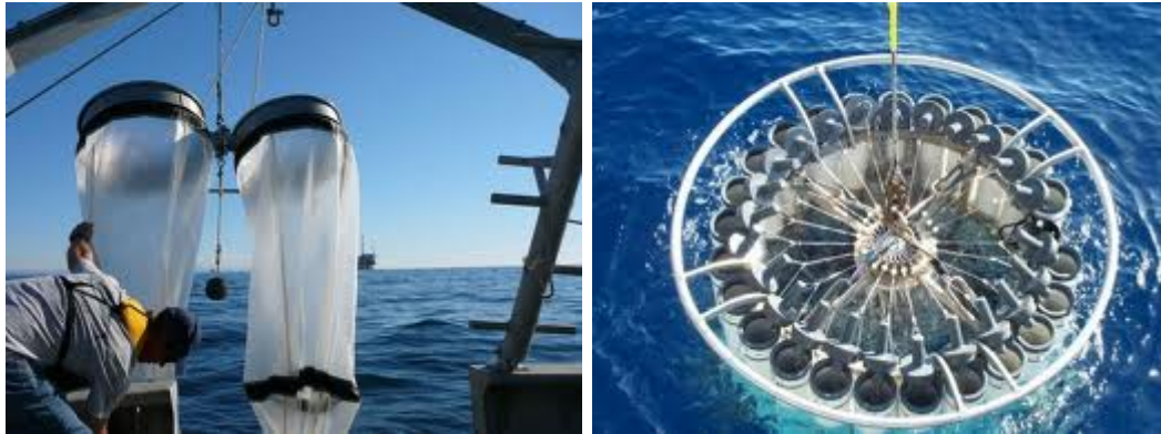
(a) Plankton tow net, 153-m pore size, 0.5-m diameter (D:L=1:3) (b) Multiple opening/closing net system
