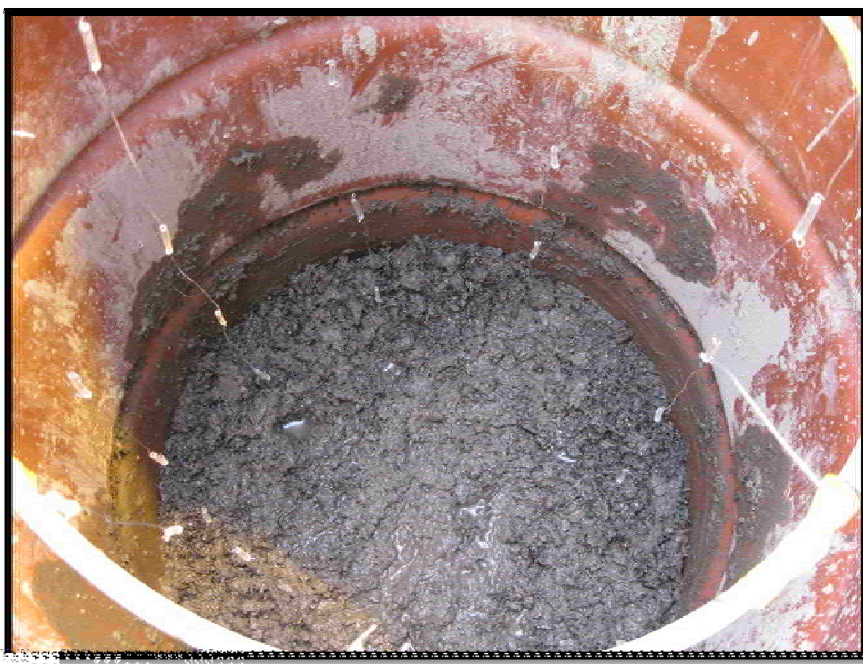
200-L reactor showing 40-SPSs placed in subsurface
