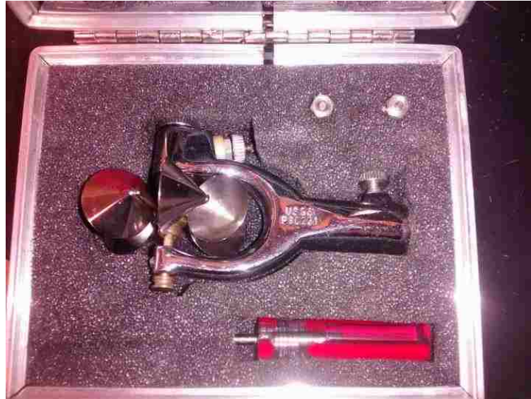
Figure 3.3. Pygmy meter used during flow monitoring.
