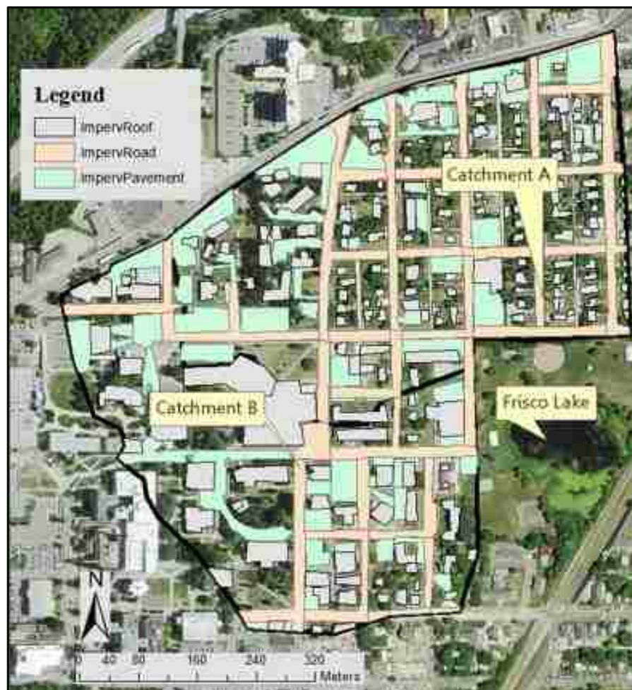
Figure D1. Delineated impervious surface land covers within Frisco Lake watershed using geospatial analysis software ArcMap 10 (ESRI).
