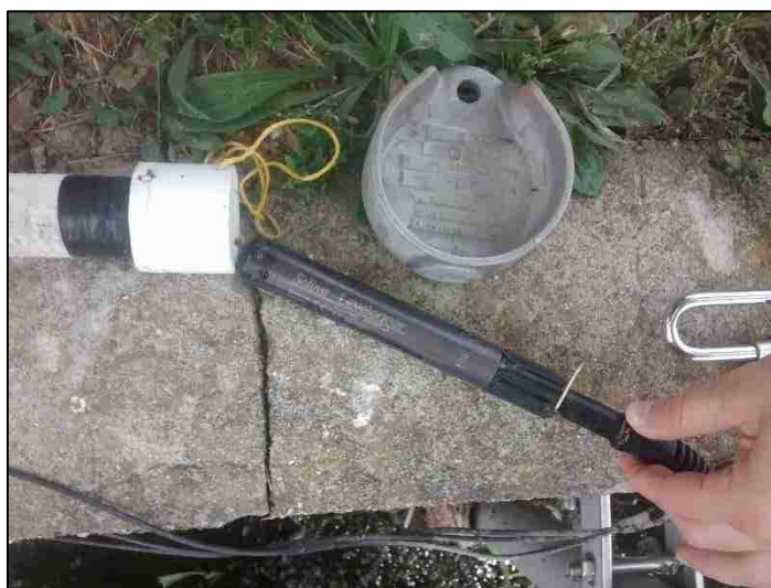
Figure B1. Levelogger, PVC stilling well, and metal monitoring well equipment.
