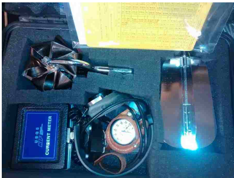
Figure 3.4. A field instrument box storing Price AA and pygmy current meters, headset, stopwatch, and linear to radial velocity conversion chart.
