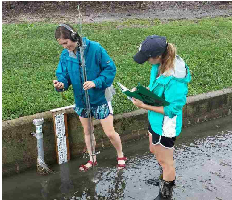
Figure 3.5. Streamflow velocity measurements are taken using Six-Tenths method.
