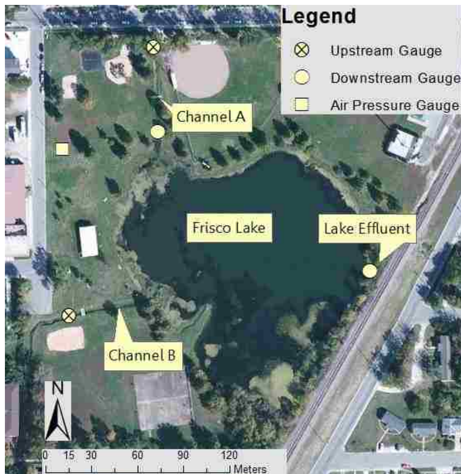
Fig. 2 Project study area with lake influents and effluent and streamflow monitoring equipment locations denoted.
