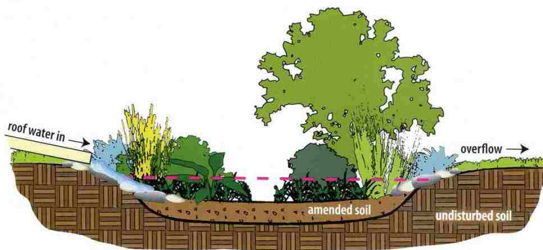
Figure 3.9. Schematic of a typical rain garden set up (after OSU 2010).
