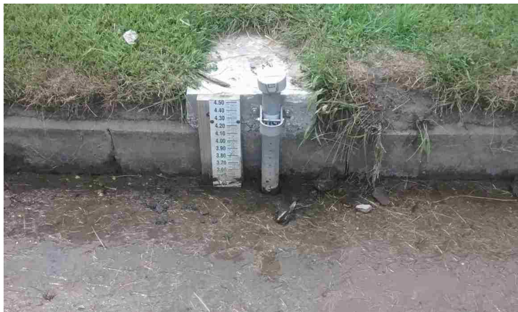
Figure 3.2. Stream gage and staff gage within a channel.
