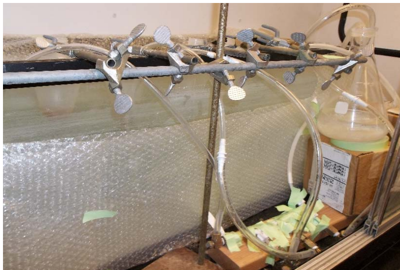
Figure 2.4: PBET Setup – View of PBET Tank with Separatory Funnels
