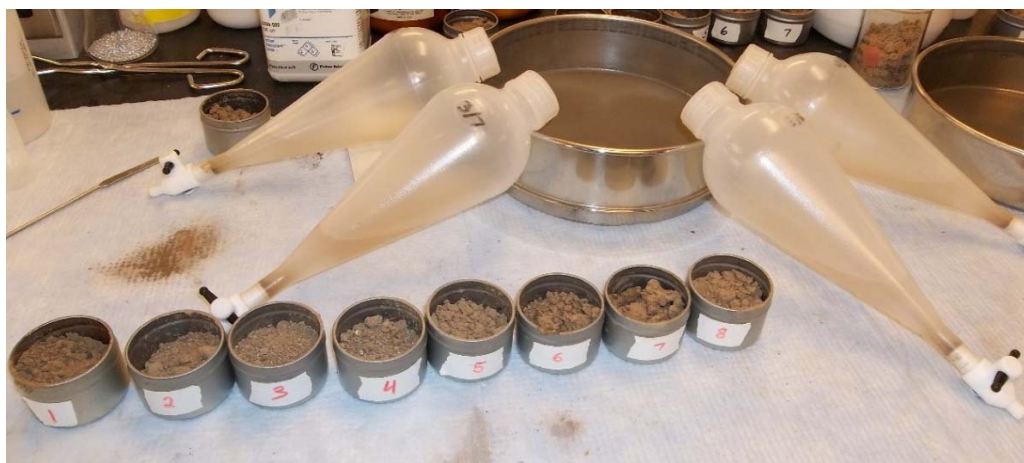
Figure 2.3: Soil Preparation for PBET
