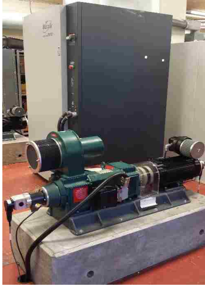
Figure 7. Motor/dynamometer experimental setup.
