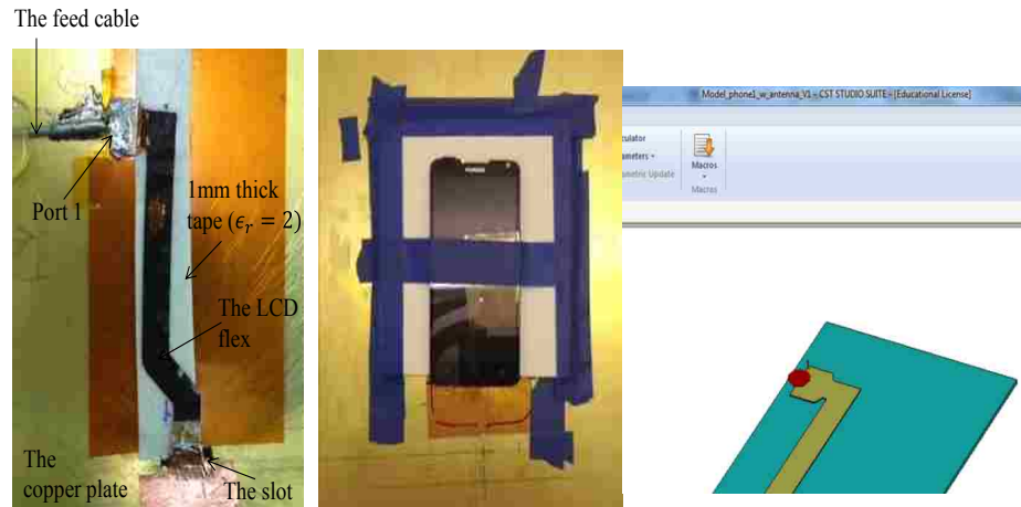
Fig. 17. (left) Bottom view and (mid) top view of the setup built for characterizing the LCD, and (right) full-wave model of this setup (the copper plate is hidden from view).
