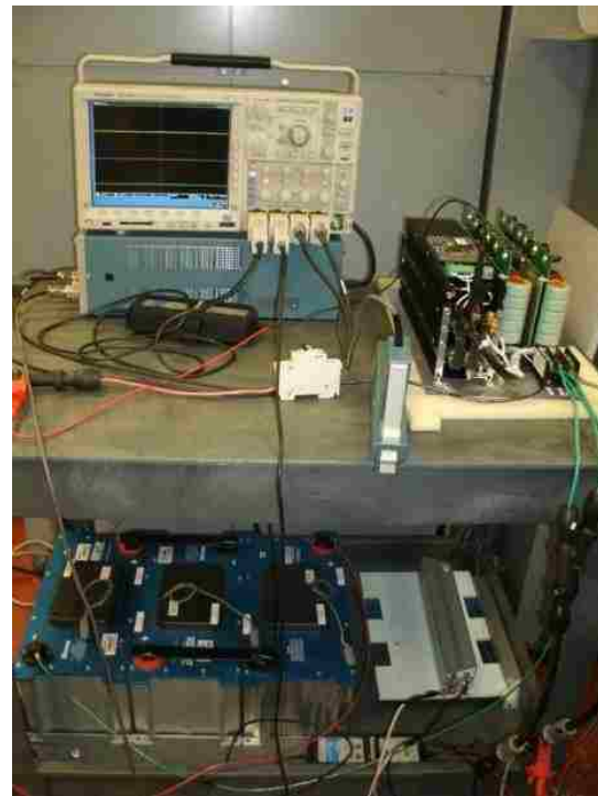
Fig. 7 (b) Bi-directional dc-dc converter and MSO4034B oscilloscope (top shelf), UCAP and 213.5\Omega load (bottom shelf)
