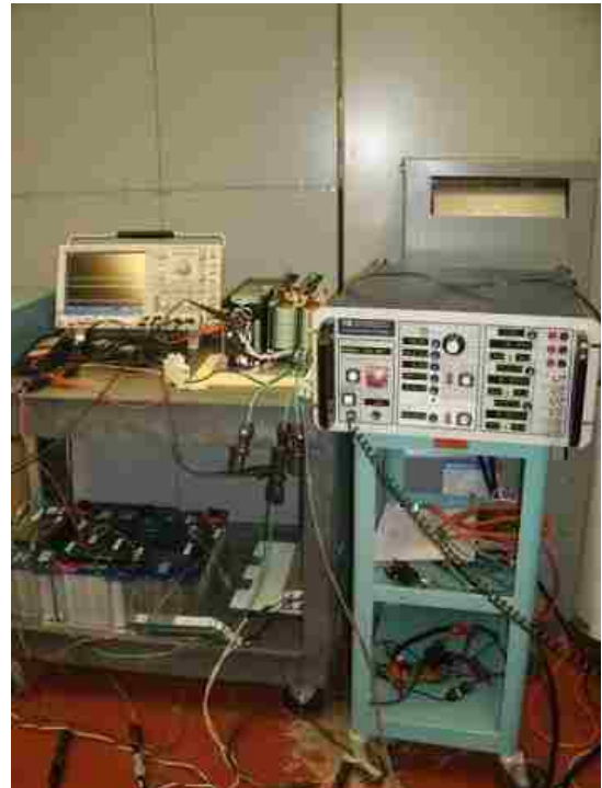
Fig. 8 (b) Dc-dc converter and MSO4034B oscilloscope (top shelf), UCAP bank with 3 UCAPs (bottom shelf) and the Industrial Power Corruptor
