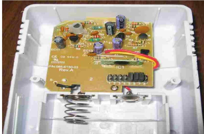
Figure 3. 1. Circuit of a doorbell used for experiment
